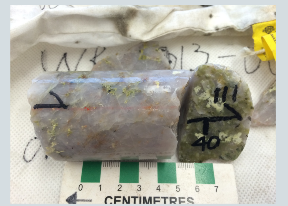
Fig. 4-B: Oriented sample of hydrothermal quartz (WR-440)
