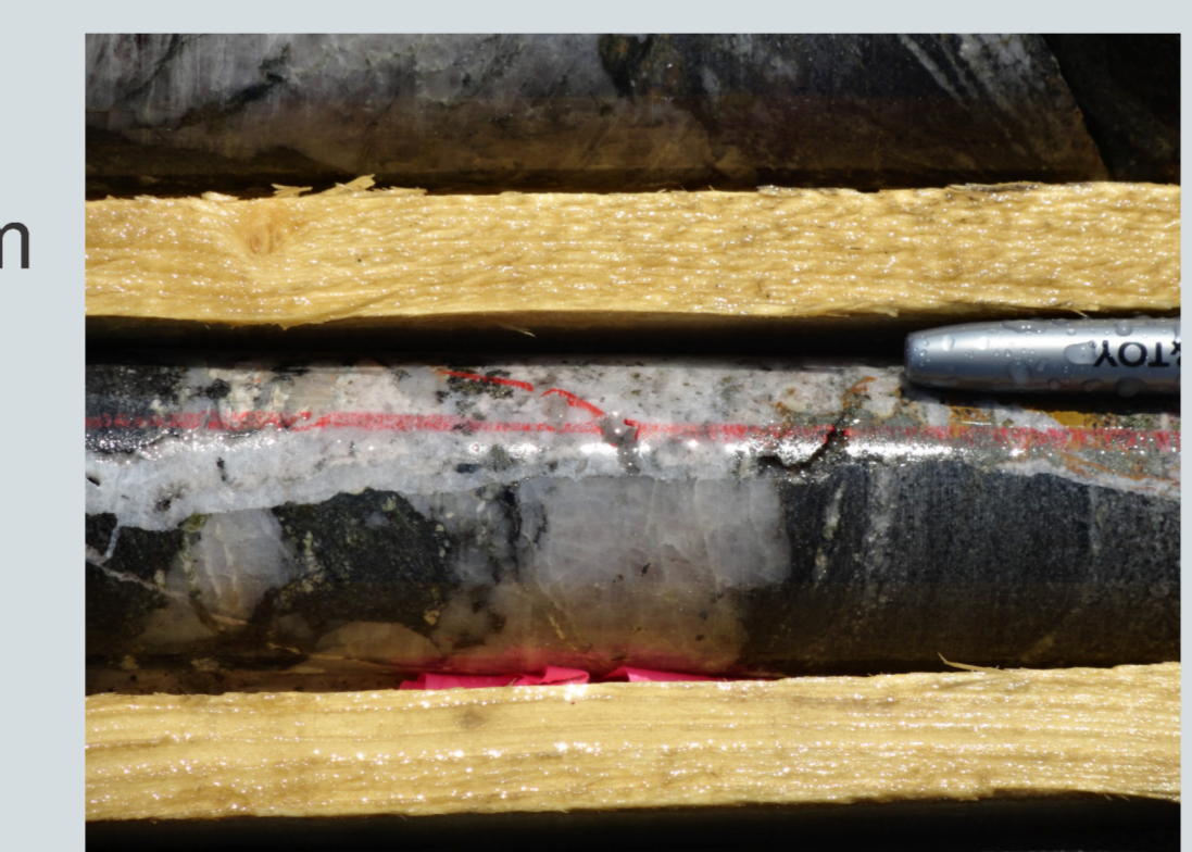
Fig. 4-E: Pelite with hydrothermal quartz cut by vuggy quartz vein (WR-440)
