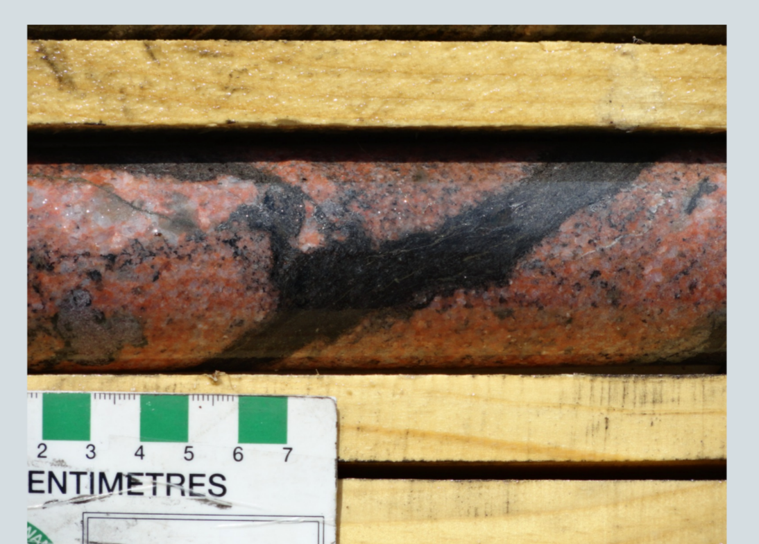
Fig. 4-D: Hydrothermal graphite vein cutting granite (WR-440)
