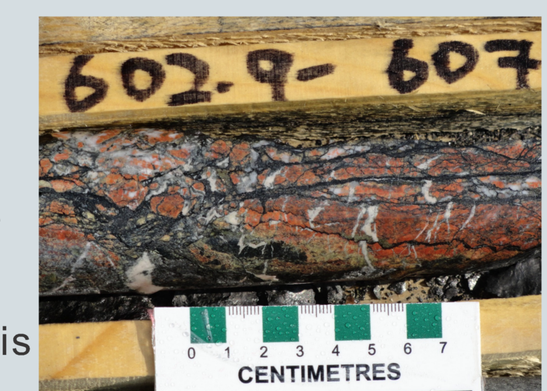
Fig. 4-C: Pegmatite cut by graphite-filled fractures (WR-440)
