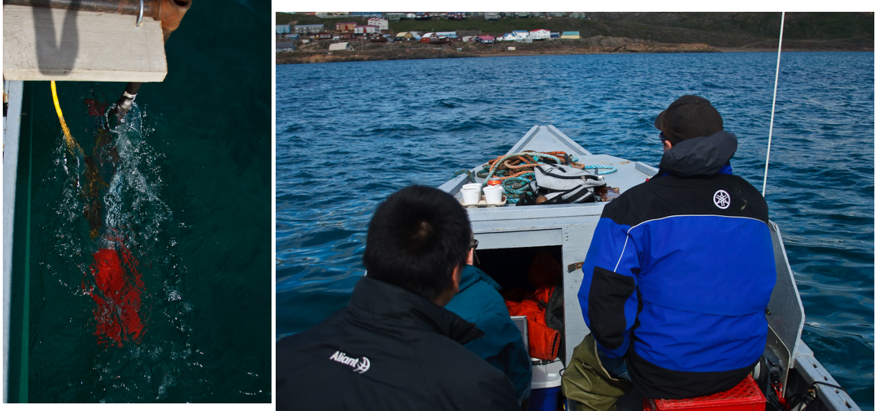
(a) Sensor mount setup with the Sidescan Sonar
