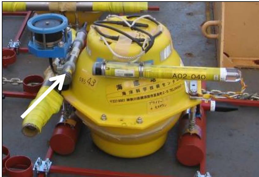
Figure 4. JAMSTEC OBS as used during expedition 2013008PGC with the additional battery pack (white arrow) at the transducer to allow for a 10 month deployment time.
