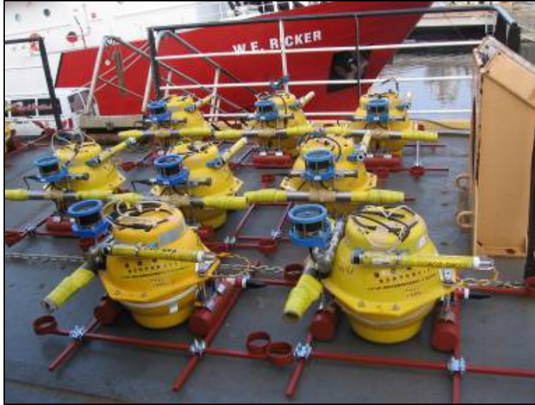
Figure 3. Image of the JAMSTEC OBSs stored on the upper deck above the lab prior to actual deployment. On this level, up to 18 OBS were stored, with the remaining OBS stored on the regular back-deck.
