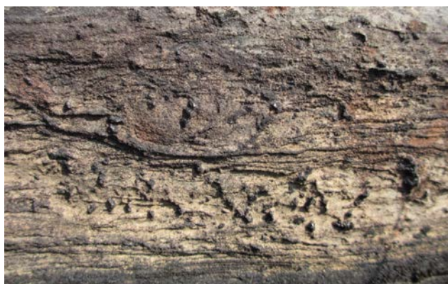
Figure 9. Dolomite stratabound iron oxide altered and veined by iron oxide. Both hematite and potentially wustite? Were observed in distinct alteration zones.
