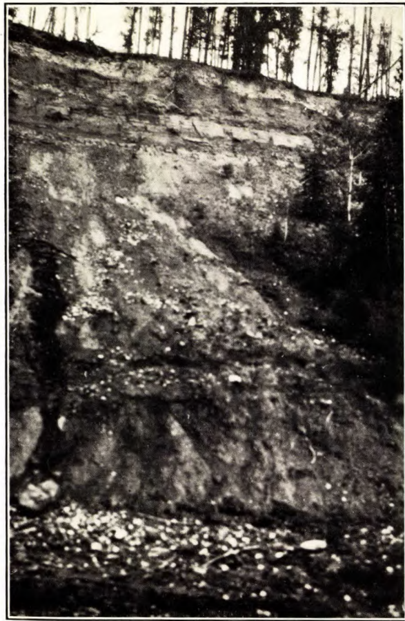
A. Typical exposure of bituminous sand on Beaver river (sec. 25, tp. 93, R. 11) showing light gravel overburden.
