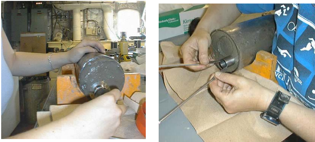
Figure 12: Taking a shear strength measurement with a Torvane (left) and a constant volume
