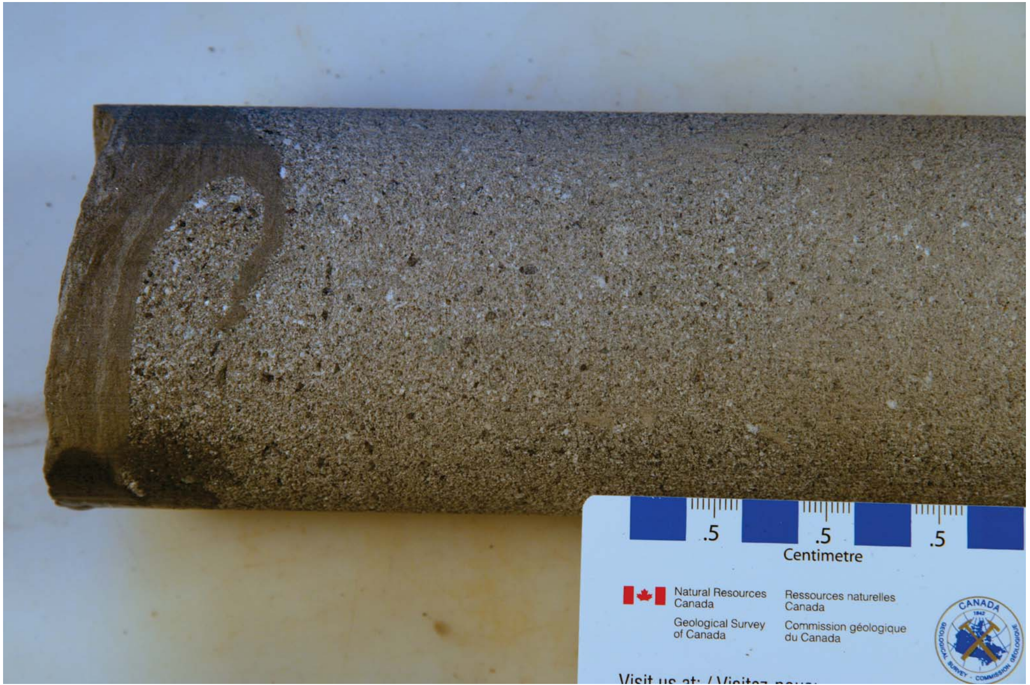
Figure 5. Sharp base and lower portion of thick bedded, well-sorted, massive, fining-upward, permeable coarse-grained sandstone bed, ~ 91 m depth, stratigraphic top to right.
