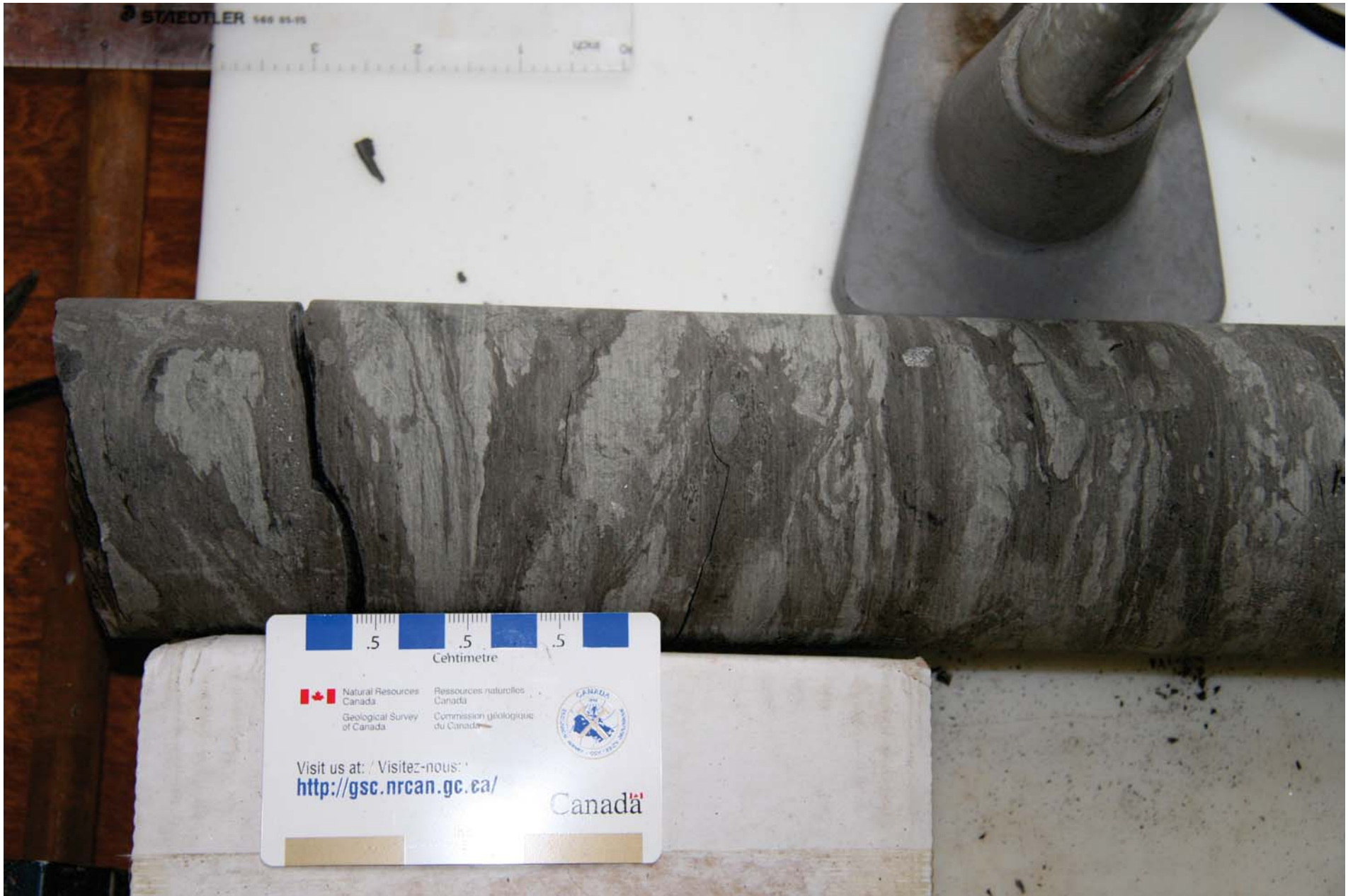
Figure 6. Thinly interbedded and burrow-homogenized dark grey siltstone and fine-grained sandstone, with abundant soft-sediment deformation, ~ 67 m depth, stratigraphic top to right.
