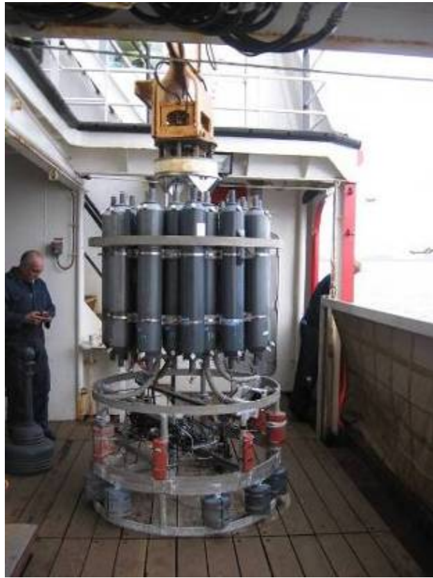
Figure 9 Water sampling rosette and CTD deployed during cruise 2012005PGC.
