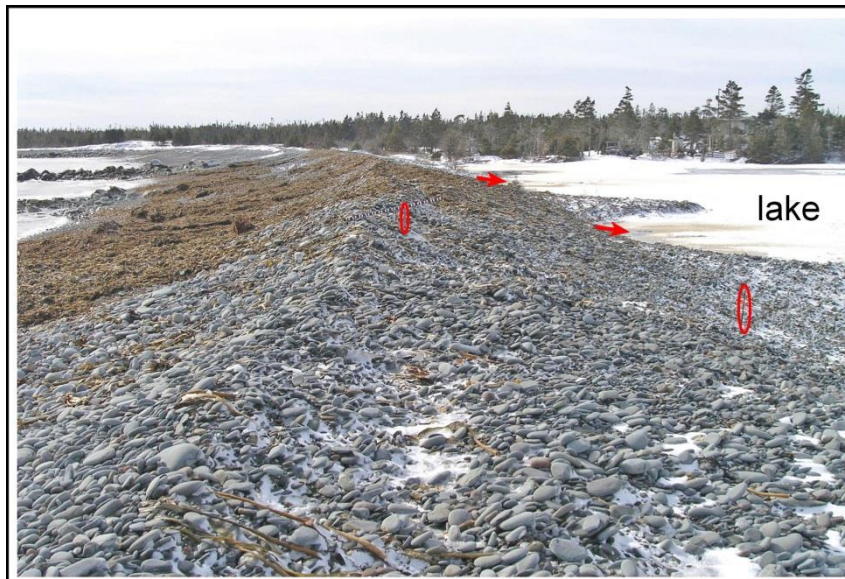
Figure 18. Miseners Long Beach: The cover of seaweed and presence of melt holes (arrows) in the lake ice provide evidence of the extent of wave overwash just west of Line 2 (line markers circled). Beach crest elevation before the storm ranged from 3.7 to 3.9 m (GD).
