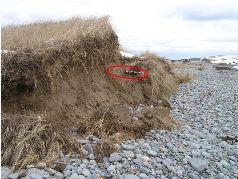
Figure 14. Lawrencetown Beach-east end: Waves scoured and overtopped the present foredune to elevations of 3.6 to 3.8 m (GD). Where the exposed foredune was higher, as shown in this photo, waves scoured the base of the dune, causing large chunks of frozen dune to break off. The graduated rod for scale is 1.5 m long.
