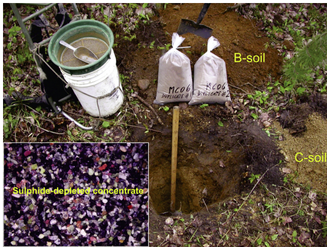
Figure 5. Typical sample pit in oxidized till in Canada. Till excavated from the B- and C-horizons of the overprinted soil profile has been piled separately to illustrate their different oxidization states. Ideally, the sample is obtained from the weakly oxidized, pale yellow-ochre C-horizon below the highly oxidized, dark red-ochre B-horizon, generally at a depth of 0.5 to 1 m. The insert shows the heavy mineral fraction of the till in which most of the original sulphide grains have been consumed by oxidation.
