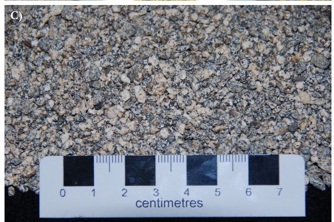
Figure 8. A) Sample site of the unconsolidated weathered Silurian-Devonian granite (grus) used for GSC blank heavy mineral samples. B) Close-up view of the blank sample material. C) Close-up view of the 2–4 mm fraction of the blank material.
