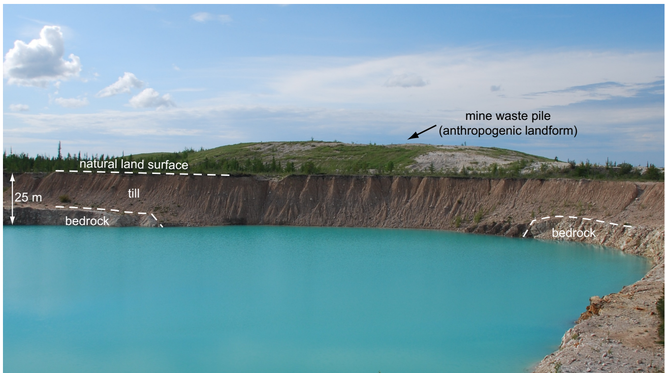
Figure 6. A till sample site in a region heavily disturbed by anthropogenic activity at the old Pine Point Pb-Zn Mississippi Valley-type mining district, Northwest Territories. Till samples were collected in a former open pit mine, below the original natural land surface (Rice et al., 2013), and away from mine waste piles, which consisted of till excavated from the former open pit, mixed with other mine debris.
