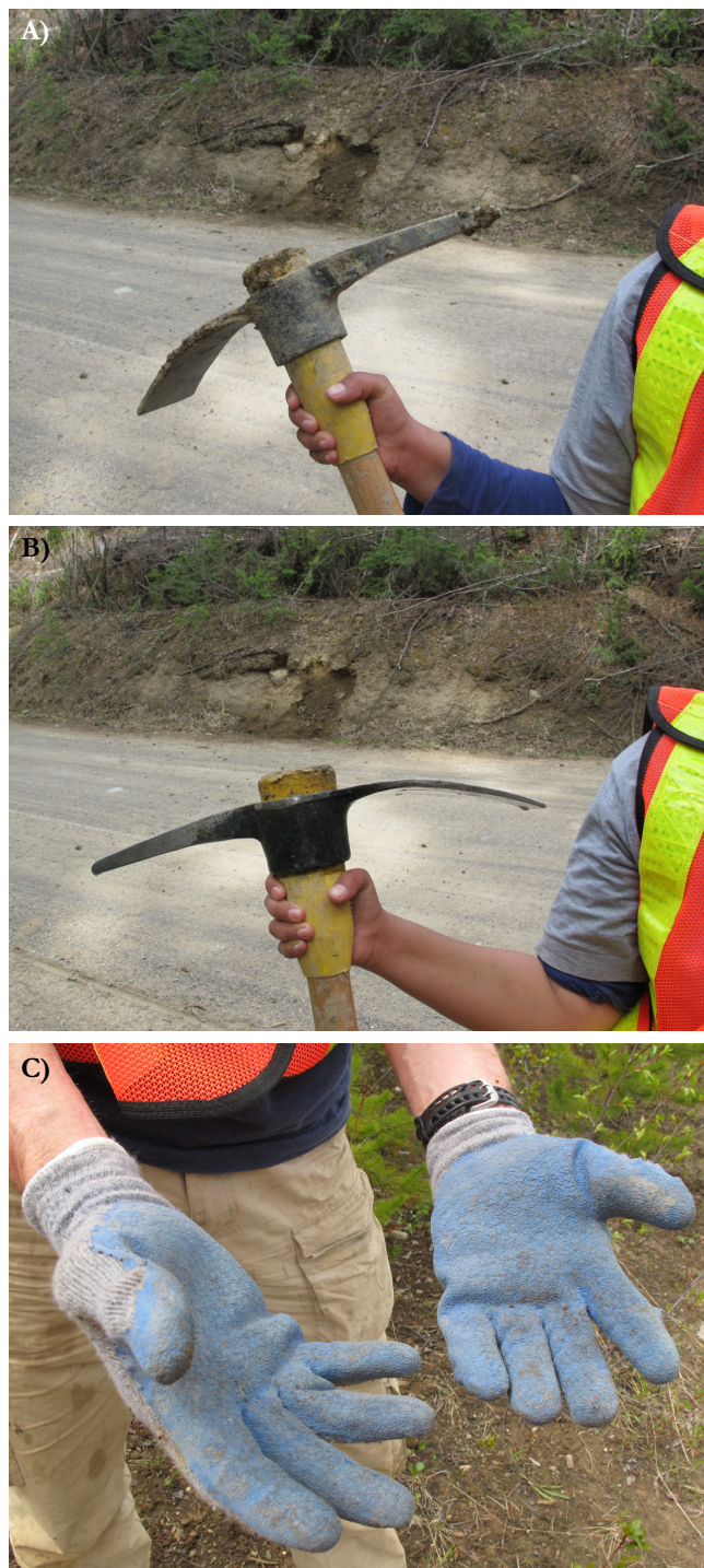
Figure 4. A) A dirty pick with sediment stuck to it after the collection of a sample, and therefore unsuitable for the collection of the next sample. B) A cleaned pick ready for the collection of a sample. C) Work gloves represent a potential source of contamination.
