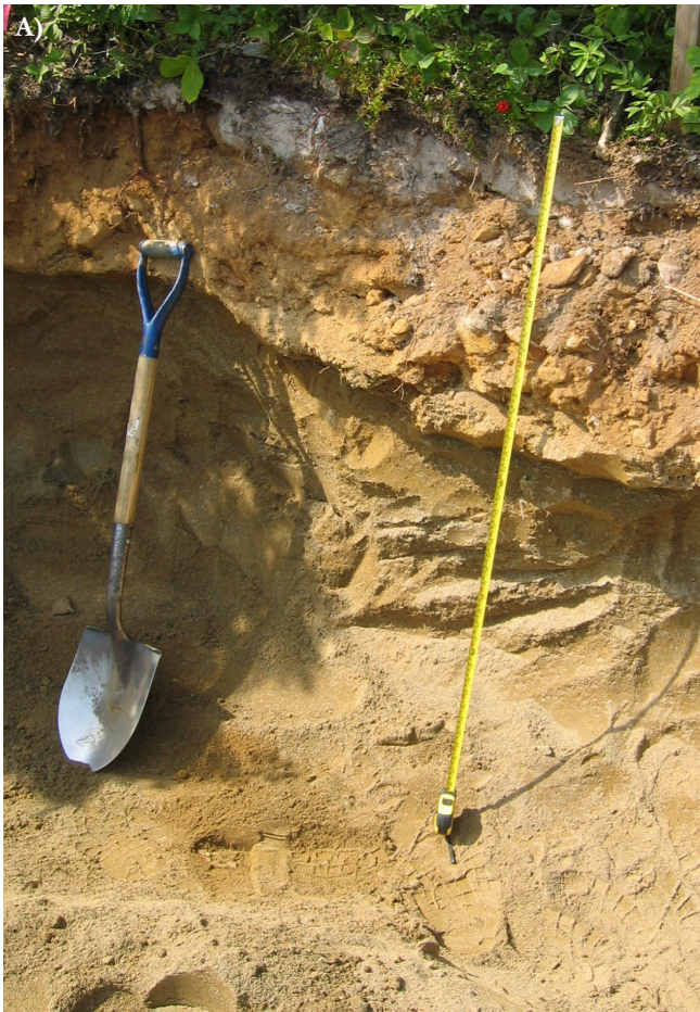
Figure 8. A) Sample site of the unconsolidated weathered Silurian-Devonian granite (grus) used for GSC blank heavy mineral samples. B) Close-up view of the blank sample material. C) Close-up view of the 2–4 mm fraction of the blank material.
