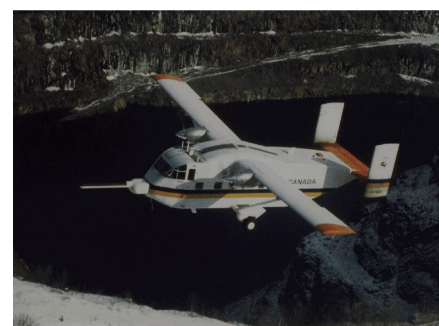
Figure 1. A geophysical survey aircraft (GSC's Skyvan) airborne radiometric survey platform, 1968-1994
