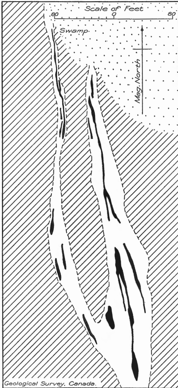
Figure 4. Northern part of schist zone on North Star gold prospect, Morton Lake area, Manitoba, showing position of quartz veins, etc. (solid black), in schist zone (blank) in massive andesite (pattern of ruling). Drift is shown by a pattern of dots.
