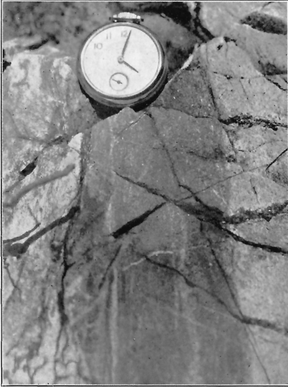
Band of richly disseminated chromite in "serpentine rock". Cut by later (white) serpentine veinlet. One wall of the band is sharp, the other gradational. E deposit.
