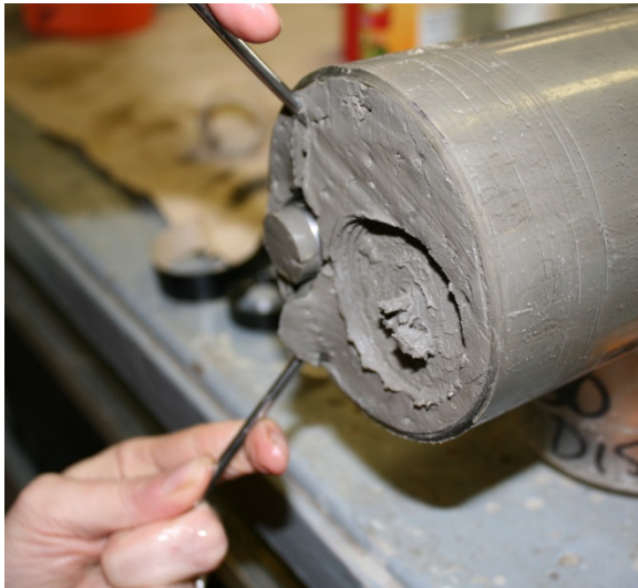
Figure 6.6 Taking a constant volume sample.
