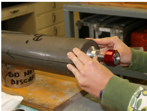
Figure 6.5 Taking a Torvane measurement.
