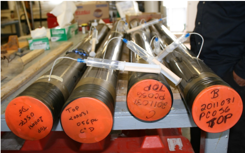
Figure 6.9 Extracting pore water samples from sediment cores.
