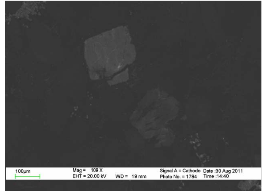
A99-2933.67-11: SEM-CL image shows two detrital Kfs grains that are of different brightness.
