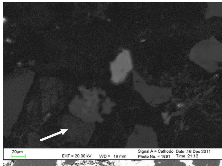
J47-5445.94-18: SEM-CL image shows weak luminescence Olig and detrital Ab (arrow).
