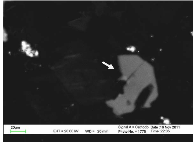
H59-3904.80-14: The diagenetic Ab overgrowth region is dark in the SEM-CL image (arrow).
