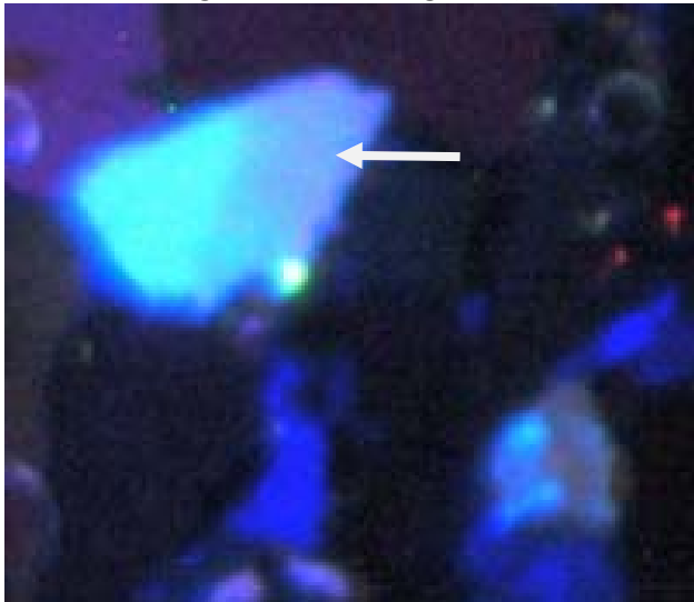
G67-2431.72-3: HC-CL image shows blue Kfs with darker zoning (arrow). This may indicate magmatic zoning.
