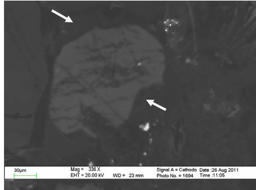
A99-2212.12-2: SEM-CL image shows an overgrowth zone (arrow points) to be dark and the core has dark CL patches.
