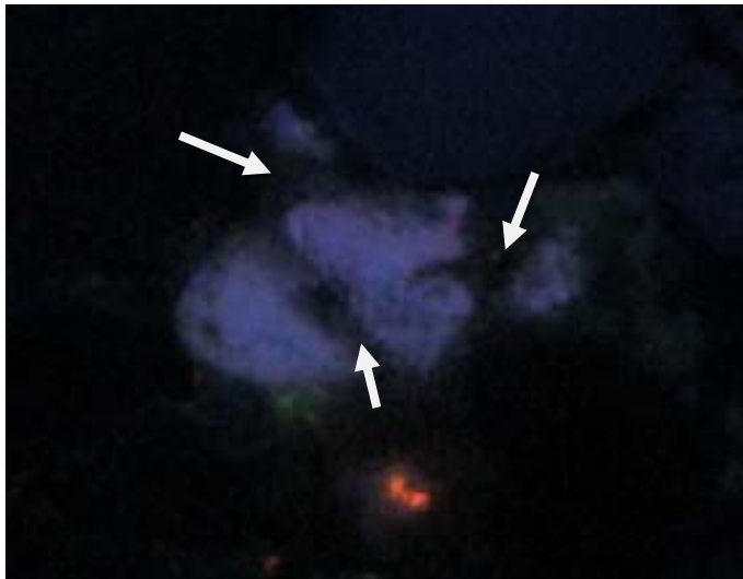
A99-3794.17-25: HC-CL image shows diagenetic Ab patches are dark (arrow) and detrital Ab is pinkish blue.
