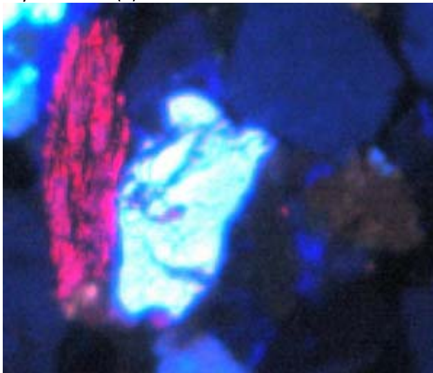
G67-2431.72-14: HC-CL image shows bright blue, blue and pinkish Kfs. Albitized area is pink.
