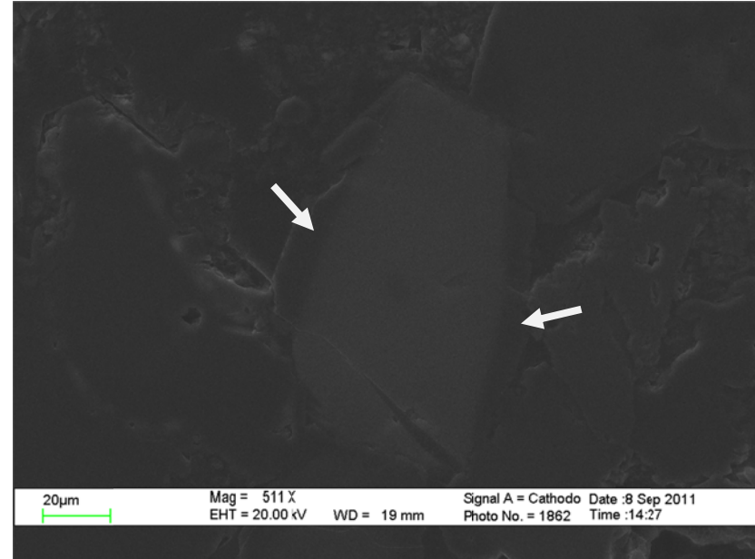
A99-2470.66-17: SEM-CL image shows the overgrowth areas (arrow) are darker than the core.
