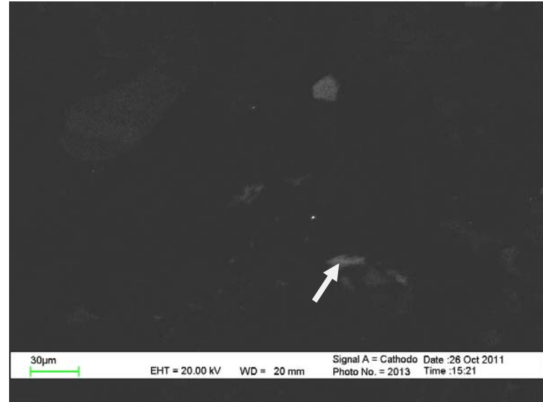
TH5-4925.84-20: SEM-CL image shows dark Ab and weakly luminescence Olig (arrow).
