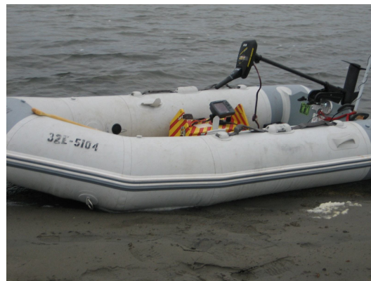
Equipment used for the depth survey of Ice Lake
