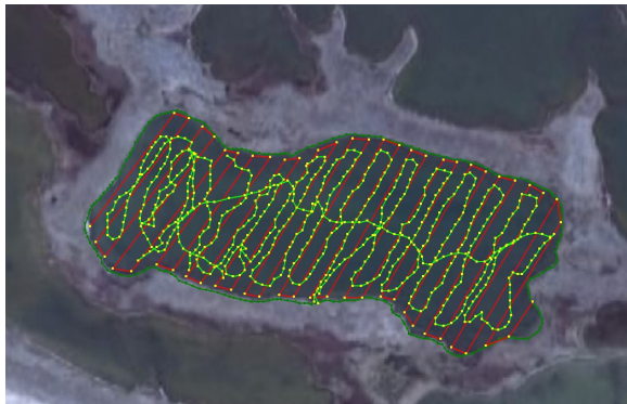
Ice Lake survey path and resulting depth model.
