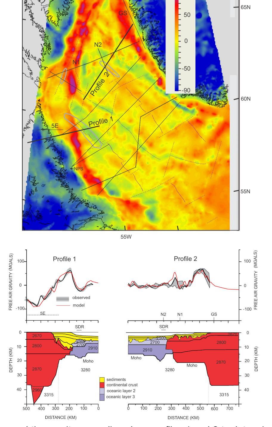
We used the gravity anomalies along profiles 1 and 2 to determine the crustal structure below the conjugate margins. The structure is constrained by seismic data, while densities are constrained by seismic velocities and sonic logs in exploratory wells; crustal densities are the same on both profiles.
