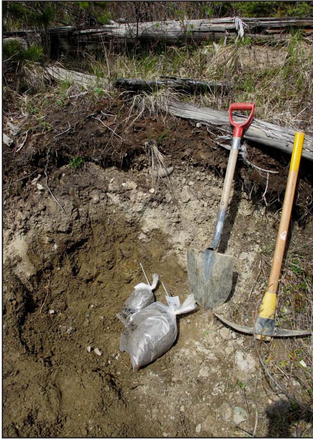
Figure 4. Subglacial till sample site (2 kg and 10 kg samples) in the Gibraltar study area. Pick for scale (110 cm). 2013-264
