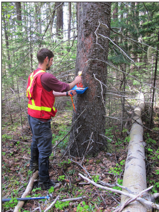
Figure 5. Collection of an Engelmann spruce ( Picea engelmannii ) bark sample as part of the biogeochemical survey in the Mount Polley study area. 2013-263
