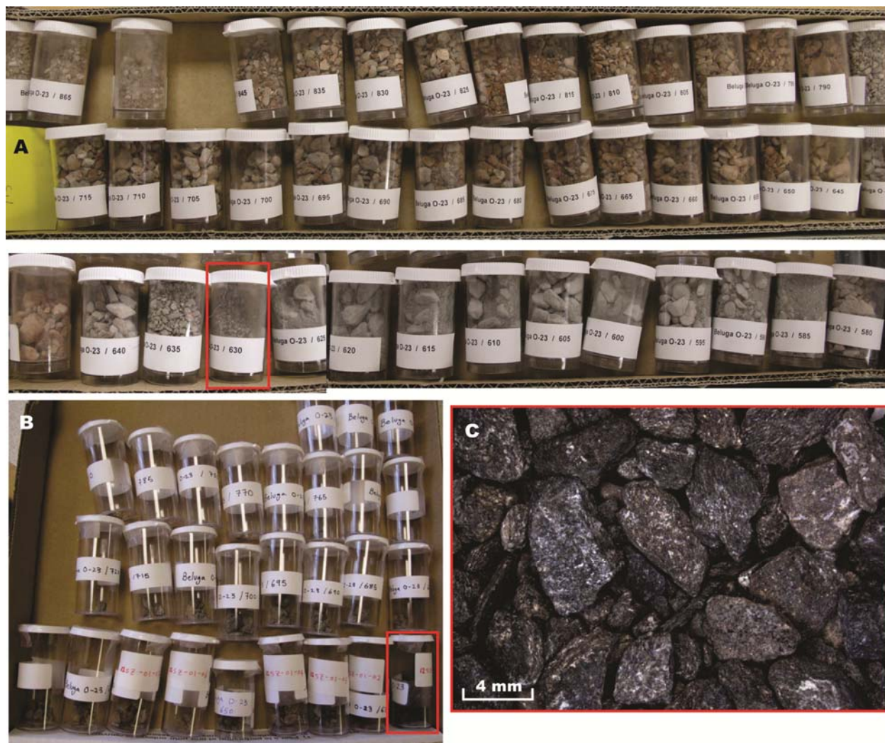
Figure 4. Part of the well cutting samples from the Beluga O-23 well. A. part of the washed well cuttings; B. possible organic-rich fragments preferentially hand-picked from 28 samples within an interval of 875-630 m; C. possible organic-rich fragment from the sample at a depth of 630 m (red box in A and B).
