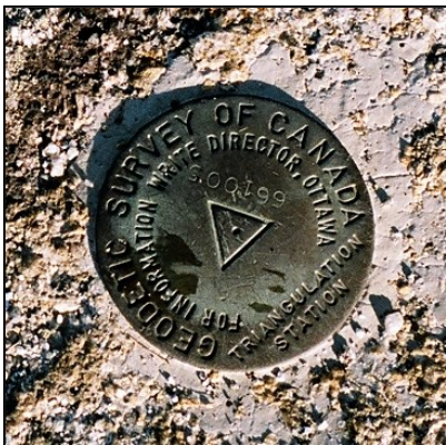
Figure 15 Triangulation station from the Geodetic Survey of Canada at the top of Position Hill:
