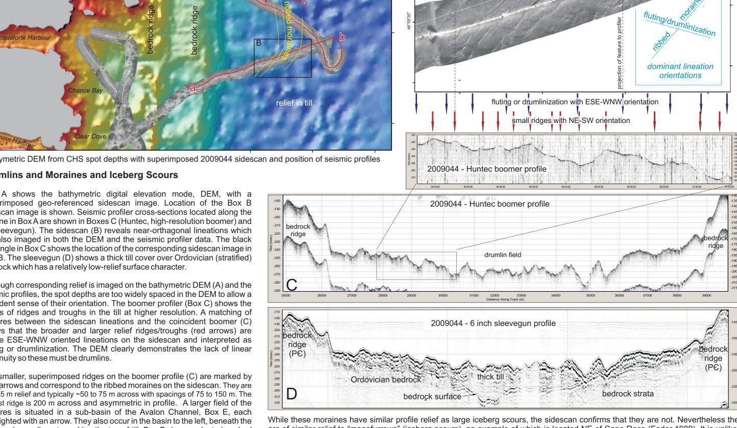
aligned with Huntec profiler section
