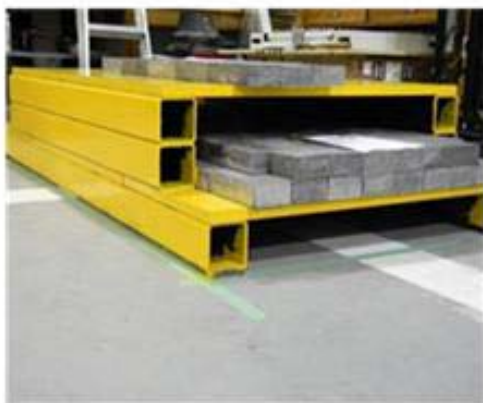
Second layer of lead installed.
