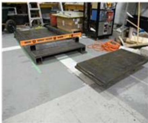
Steel plates arrive – start to build a multi-layer cosmic-ray tower.
