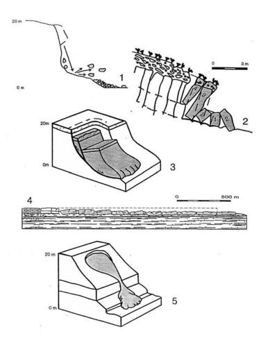
Figure 1. Mode of movement: 1) fall, 2) topple, 3) slide, 4) spread and 5) flow. Broken lines indicate the original ground surface. Displaced material is shaded. Scales are arbitrary (WP/WLI, 1993a).
