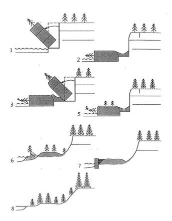
Figure 3. Topples in different states of activity: 1) active, 2) suspended, 3) reactivated, 5) inactive/dormant, 6) inactive/abandoned, 7) inactive/repaired (short term) or inactive/stabilized (long term), 8) inactive/relict. (States 5 to 8 are subsets of inactive)
