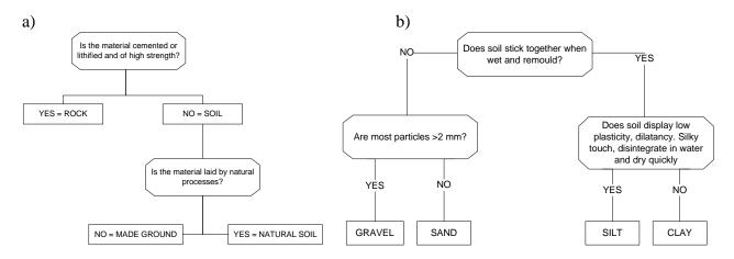
Figure 2. Flow charts for the identification and classification of soil: a) to differentiate rock from made ground from natural soil, b) to differentiate gravel, sand, silt and clay (Cruden and Couture, 2011).
