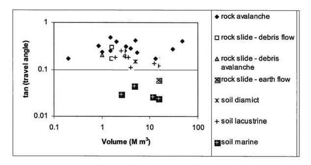
Figure 4. Volume versus tan of the travel angle for 31 Canadian Cordilleran landslides in various materials (Geertsema and Cruden, 2008).
