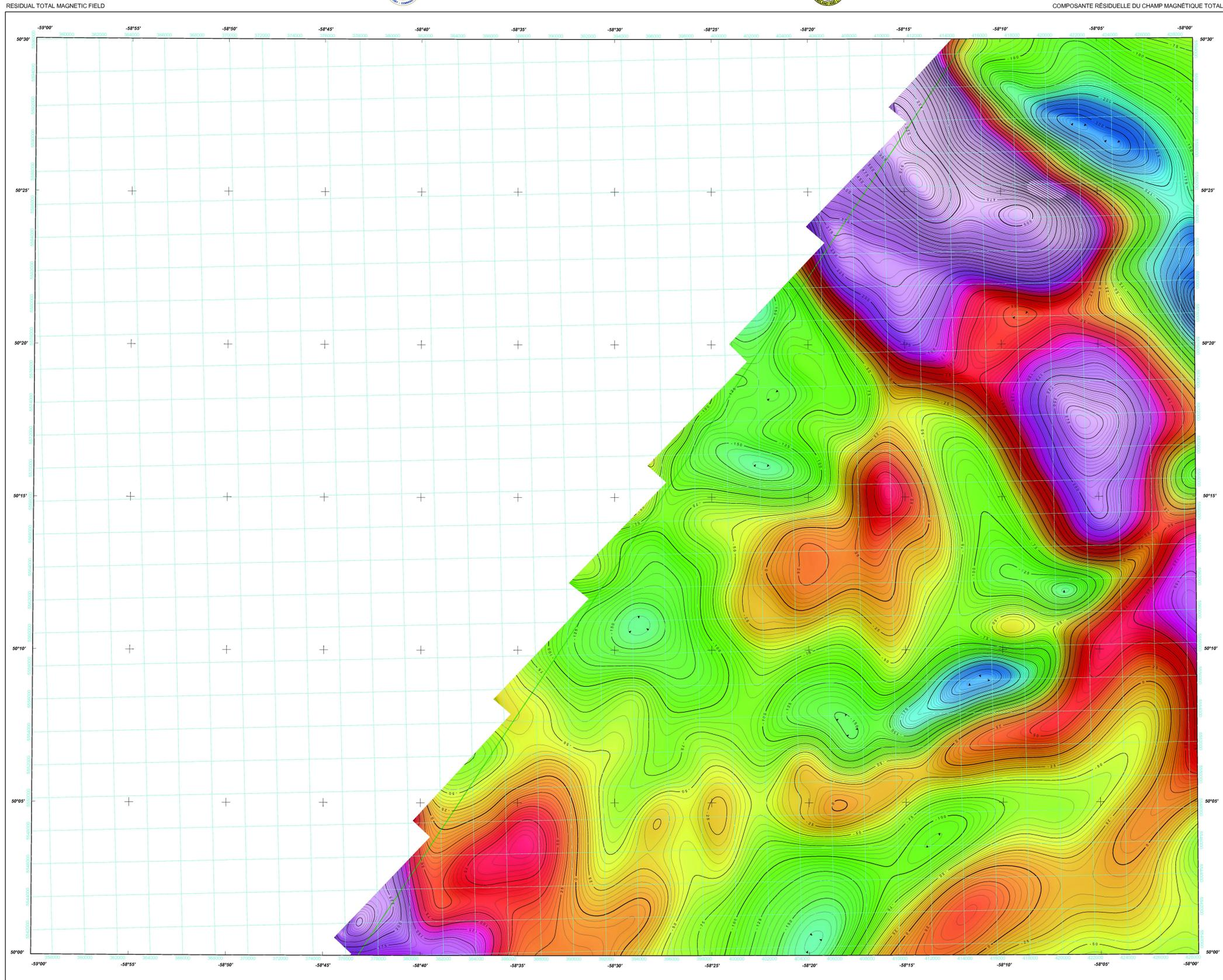
Residual Total Magnetic Field. This map of the residual total magnetic field was compiled from data acquired during an aeromagnetic survey carried out by Goldak Airborne Surveys and Terraquest Airborne Geophysics Ltd. during the period from June 8 to October 4, 2012.
