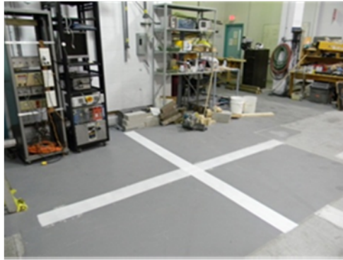
Area cleared, floor painted, coordinate system laid down.
