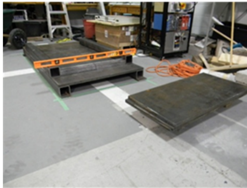
Steel plates arrive – start to build a multi-layer cosmic-ray tower.
