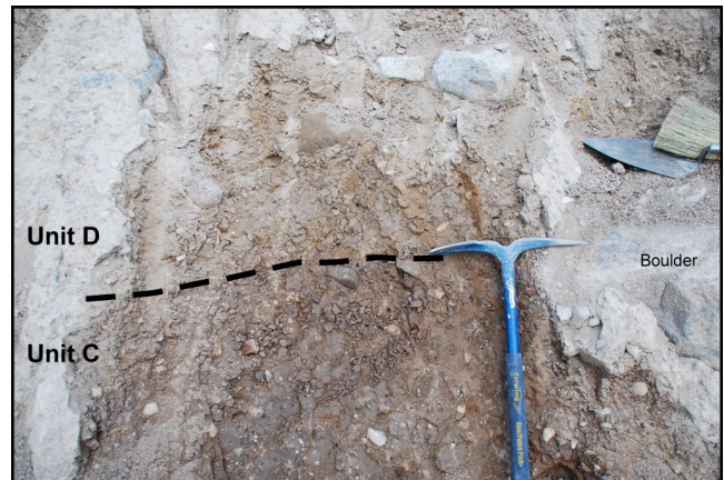
Figure 7. Sharp planar contact between till units C and D, showing the subtle differences in till colour and fissility. Boulders occur along this contact, with the tops of the boulders typically faceted and striated. Handle of pick is approximately 60 cm long. Photograph by R.C. Paulen. 2013-004
