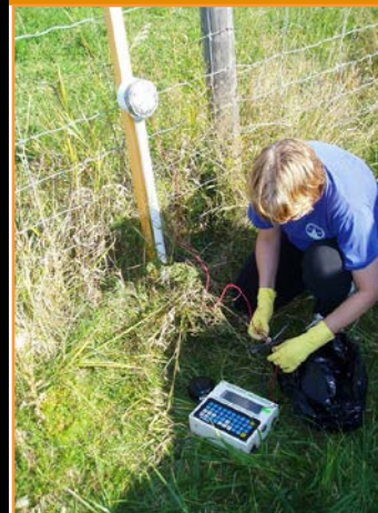
Measuring current in a buried pipeline.
