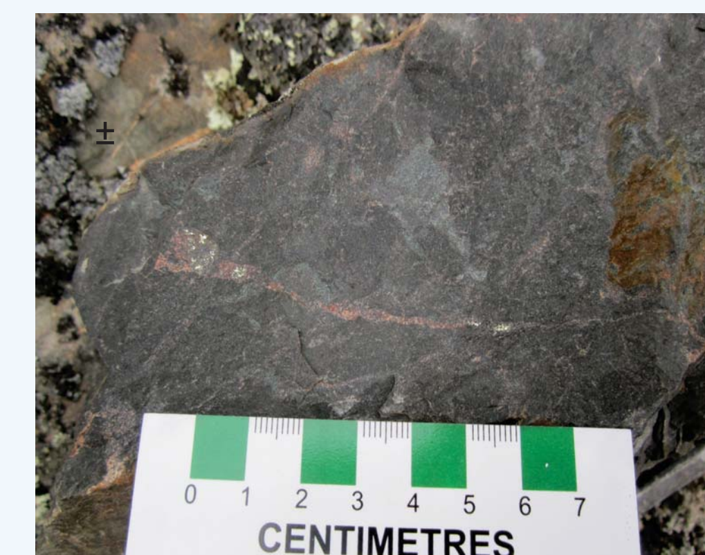
Fig. 15: Pyrite-bearing, potassium feldspar veinlets cross-cutting the main phase of amphibole-magnetite alteration. Sample 10CQA-562
