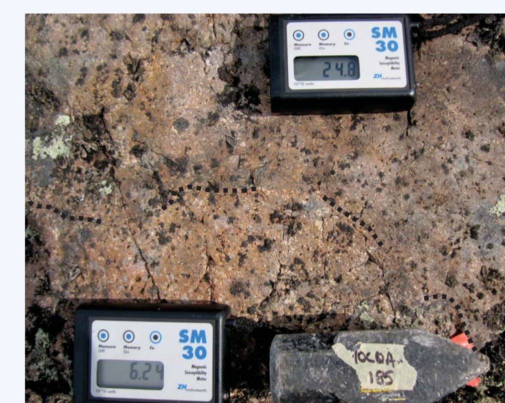
Fig. 8: Two generations of felsic feldspar porphyry dykes. The older, medium-grained feldspar porphyry (top) has amphibole-magnetite alteration, as highlighted by its greater magnetic susceptibility. Station 10CQA-185.
