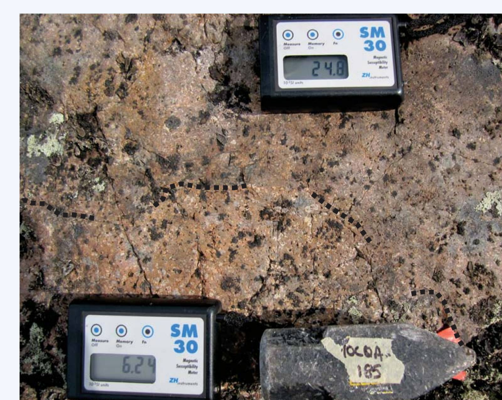
Fig. 8: Two generations of felsic feldspar porphyry dykes. The older, medium-grained feldspar porphyry (top) has amphibole-magnetite alteration, as highlighted by its greater magnetic susceptibility. Station 10CQA-185.
