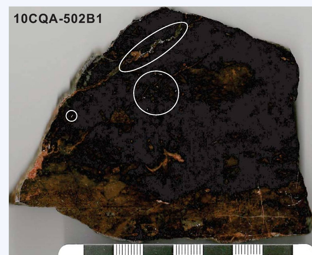
Fig. 4: Polished slab of the localized heterolithic breccia, containing intensely altered felsic porphyry clasts set in an amphibole-magnetite cement. Pyrite and arsenopyrite grains (circled) are disseminated throughout and in K-feldspar-quartz veinlets.
