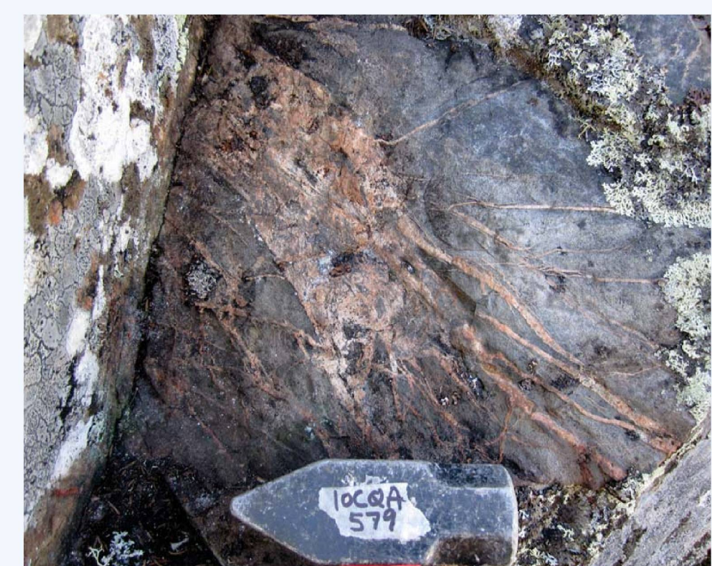
Fig. 16: Pocket of intense, K-feldspar±magnetite veins and breccia. Preliminary observations indicate that the intensity of the veining correlates with increasing U concentrations.
