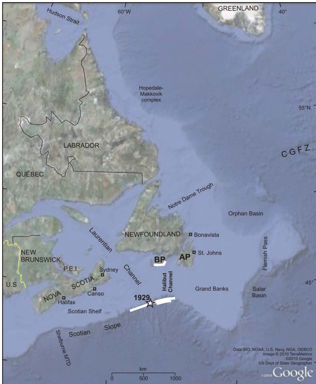
Figure 12. Map of the southeastern Canadian continental margin. White star shows the 1929 M 7.2 earthquake epicentre; associated white line shows the along-slope failure extent of the Grand Banks landslide (thicker line for the section with the greatest failure volume, e.g., Mosher and Piper, 2007). White line along the coast of the Burin Peninsula (BP) shows the extent of the most severe tsunami damage in 1929. Other abbreviations: AP, Avalon Peninsula; CGFZ, Charlie Gibbs Fracture Zone; MTD, mass-transport deposit.
