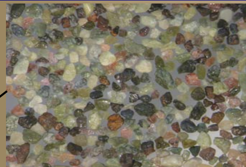
Sample 11PMA-038A-1 20% Epidote (0.25-0.50 mm)
