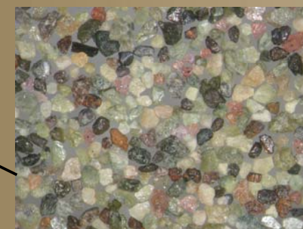
Sample 11PMA-029A-1 60% Epidote (0.25-0.50 mm)
