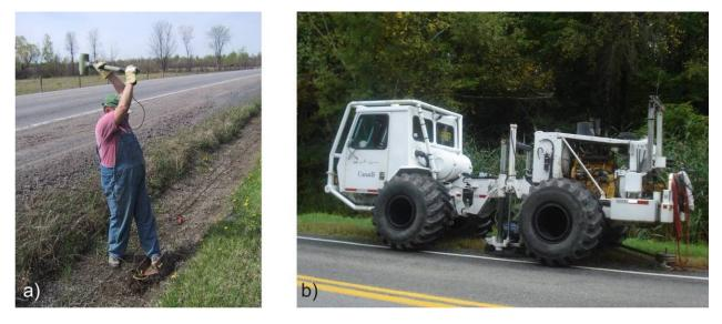
Figure 2.1.2-4. Examples shear wave seismic sources. a) Sledgehammer hitting I-beam dug into the ground. b) Large vibrating source: IVI (Industrial Vehicles International, Inc) "Minivib" vibratory source.
