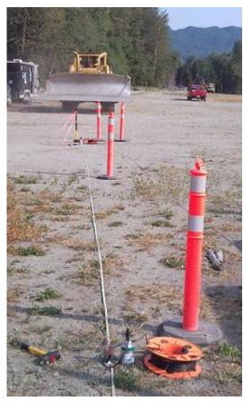
When using 1 and 2 Hz geophones in a cylindrical case (Figure 2.2.2-3), the weight of the geophones alone is adequate for coupling the receivers to the ground. The geophones must be level and set flush to the ground surface. In some situations removing the top few centimetres of loose or organic material is necessary. Smaller, higher frequency geophones usually have spiked cases that are pressed into the ground, which can present a problem in very hard or frozen soils.
