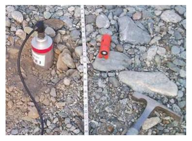
Figure 2.2.2-3. SASW receiver (1 Hz geophone).
