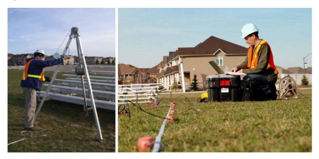
Figure 2.2.3-1: Typical setup of an MASW survey line in the field. Left side shows a seismic weight drop used as the source. Right side shows a series of geophones planted in the ground at regular spacings, and measurements are recorded with a seismograph attached to a laptop.
