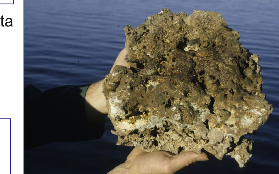
Fig 13. Sample of oil-coated Scott Trough carbonate crust collected during the Pisces IV 1985 dive.
