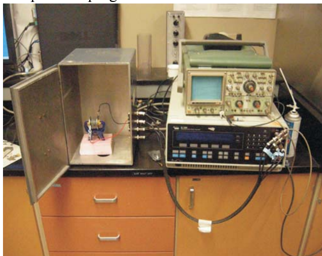
Figure 18: Solartron 1260 Frequency Response Analyzer set up to measure rock electrical impedance spectrum.
