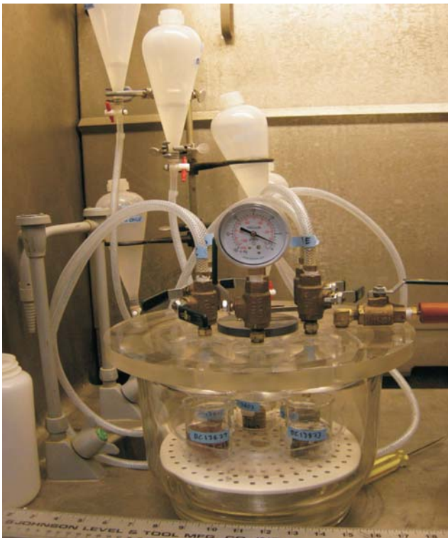
Figure 3: Chamber for vacuum impregnation of 5 subsamples.
