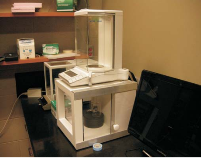
Figure 4: The immersed mass ( m_i ) of a sample being measured by suspension in a beaker of water below a balance, using a laboratory-designed Jolly balance.
