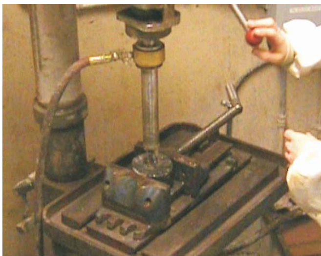
Figure 1: Drilling 2.5 cm diameter subsample cores from a hand sample or exploration core.
