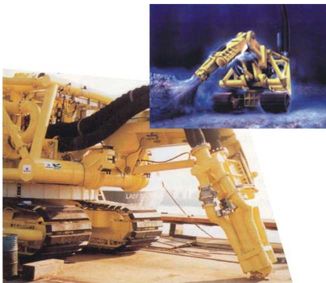
Figure 3. Photograph and artistic operating illustration (inset) of the Nam 1 seabed mining device developed for Namibian Minerals Corporation for deep water diamond mining off Namibia.
