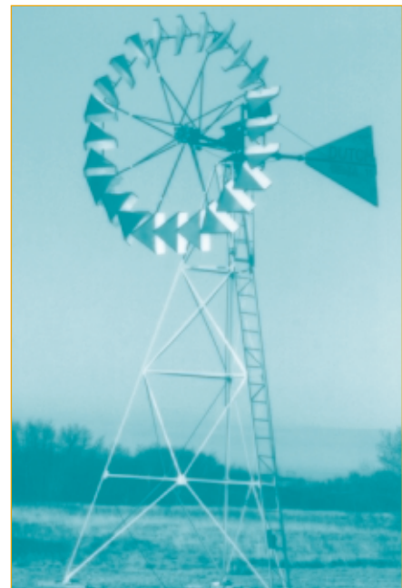
▲ Mechanical water pumping system.
