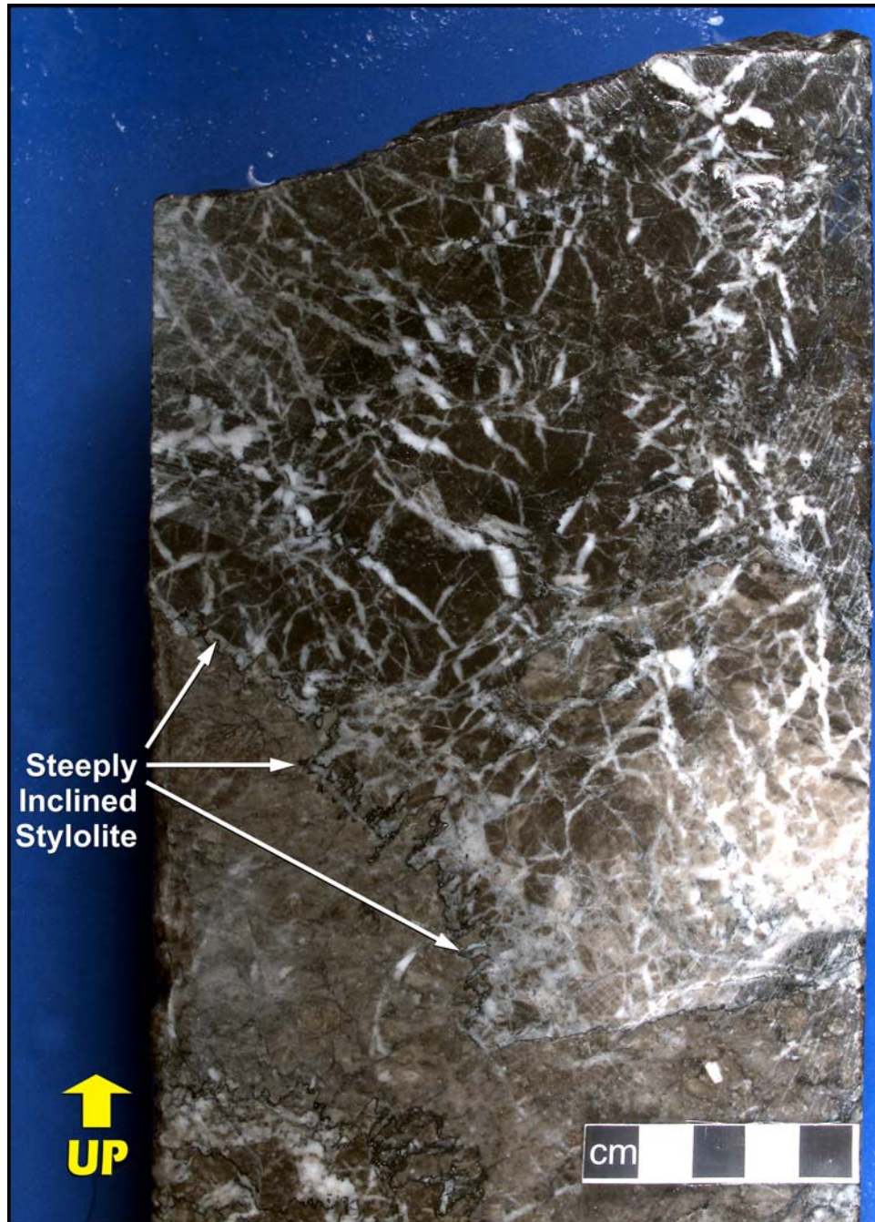
Another interpreted thrust fault in the Blue Fiord Formation, from the same well as the core piece illustrated in Figure A14 . In this case, a bitumen-infilled, steeply inclined stylolite marks the trace of the fault. Note the intensive fracture-brecciation of rocks in the hanging wall. These fractures are also infilled by white calcite cement. Photograph taken of a wetted core surface. W. Bent Horn I-01, 10685.45 ft.
