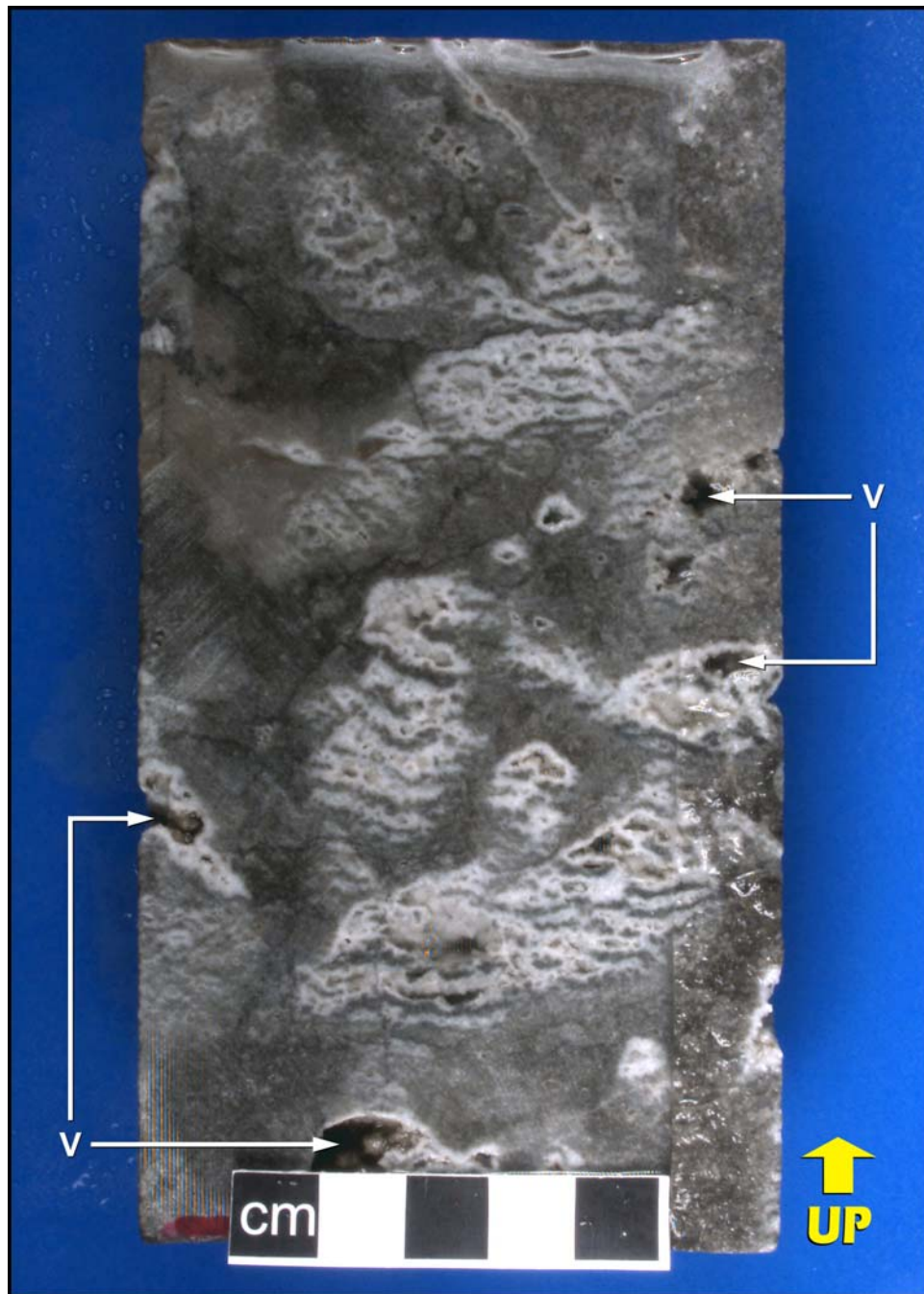
Core photograph illustrating patchy zebroids with horizontal to subhorizontal internal orientations. The core contains some open zebroid pores, partially infilled by crystals of white saddle dolomite, as well as some open dissolution vugs (V). This core interval has a measured porosity of 5.7% and a K_{max} of 0.83 mD. Photograph taken of a wetted core surface. Muscox D-87, 2087.15 m (Full Diameter Piece 37).
