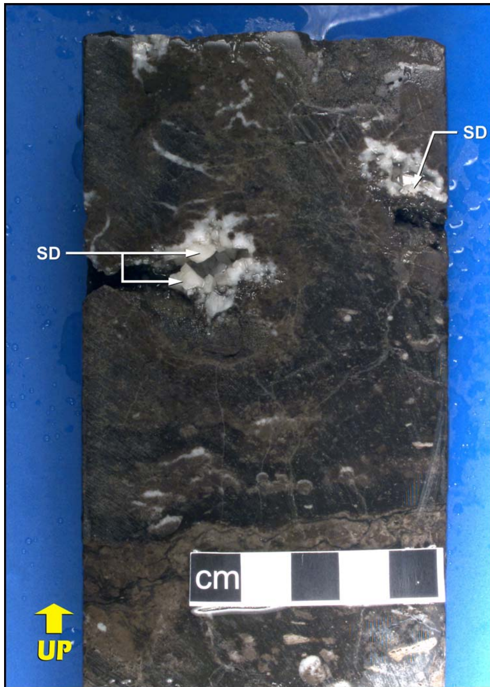
Core photograph illustrating large vugs of dissolution origin, partly infilled by crystals of saddle dolomite (SD), in a dolostone. This core core piece is from the full-diameter segment that has the highest measured porosity (13.8%) and K_{max} (50.40 mD) of any interval in the well. The large vugs are interpreted to be a major contributor to the high permeability. Photograph taken of a wetted core surface. Parker River J-72, 1002.16 m (Full Diameter Piece 1).
