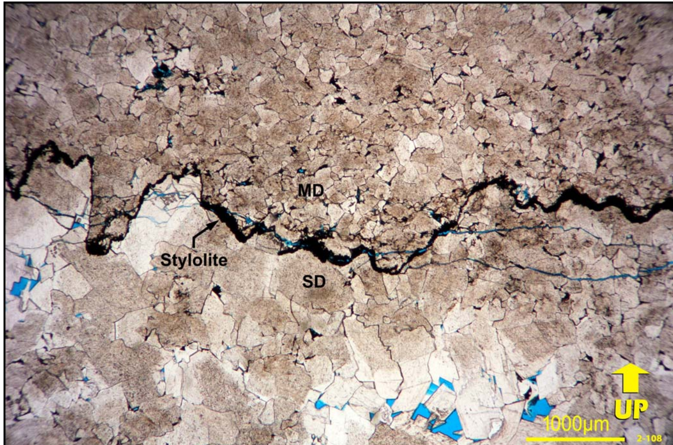
Photomicrograph of a horizontal stylolite cutting both matrix replacement dolomites (MD) and saddle dolomite (SD) infilling a zebroid pore. This relationship indicates that the final phase of stylolitization followed both matrix replacement dolomitization and saddle dolomite cementation. Photomicrograph taken using plane-polarized light. Muscox D-87, 2073.76 m.
