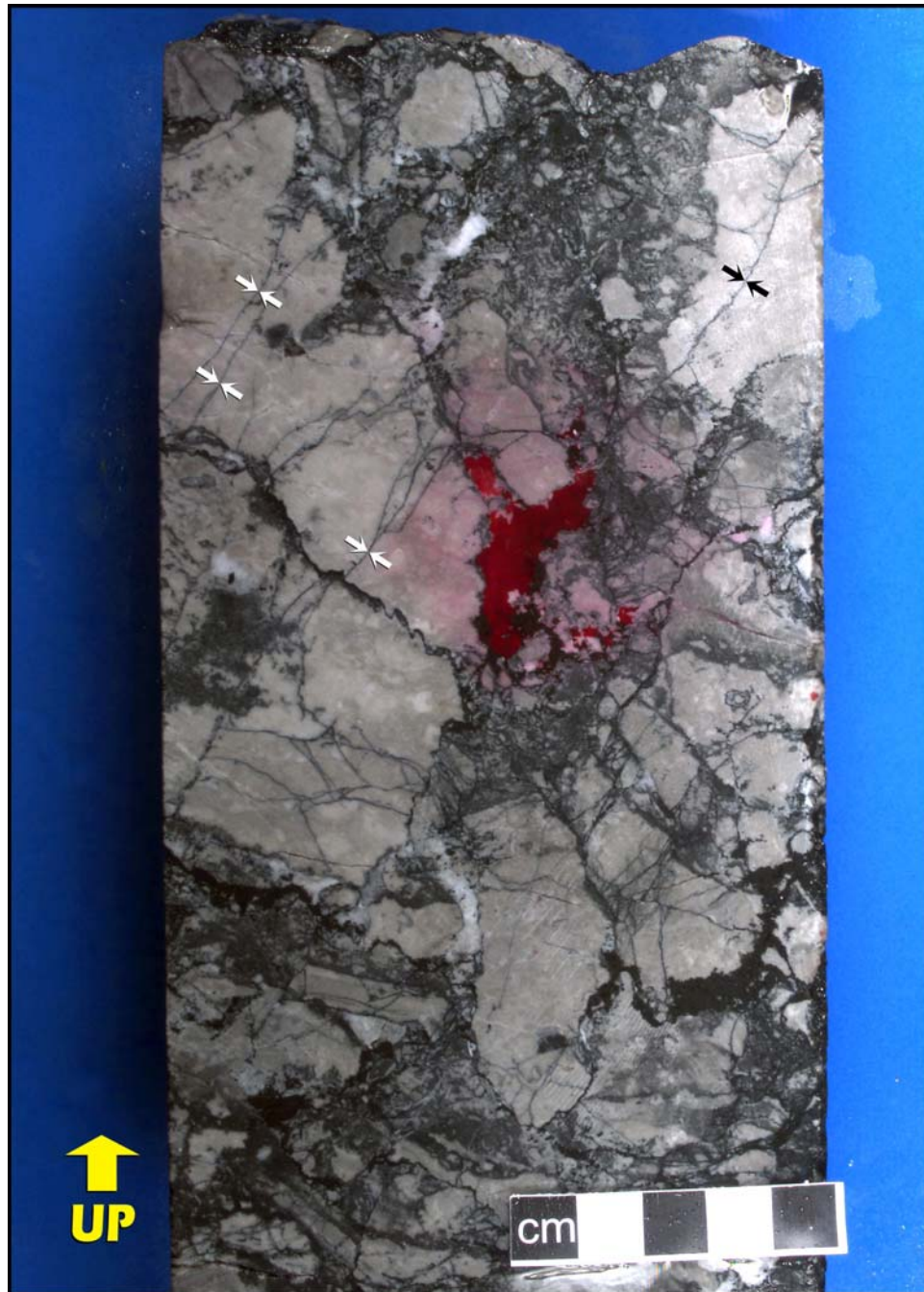
Core photograph of a matrix-rich clast-supported chaotic dolobreccia, but with some aspect of crackle and mosaic breccias. The pore sheltered beneath breccia clasts near the centre of the photograph is fringed by fine unstained white saddle dolomite cement crystals and is infilled by later Alizarin-Red S stained calcite cements. Bitumen infills narrow fractures (arrows) confined to the breccia clasts. The general lower-left to upper-right alignment of the more elongated narrow fractures in the breccia clasts suggests that fracturing followed brecciation. Photograph taken of a wetted core surface. Kusrhaak D-16, 12020.05 ft.
