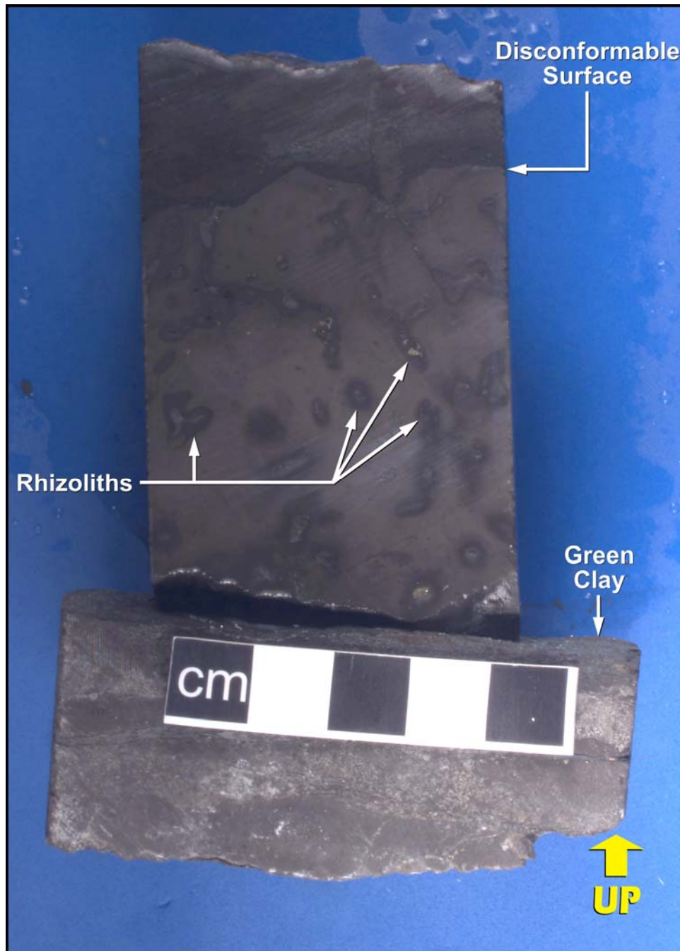
Core photograph illustrating the rooted zone in a paleosol that caps the lower succession of the upper core interval in the Parker River J-72 well. In ascending order, this photograph shows a thin interval of illuviated green clay (above the scale bar), a 4.5-cm interval containing rhizoliths (root traces) lined with dark-coloured cutans, and a 1.5-cm homogenized interval above a disconformable surface in the paleosol. The transgressive surface caps a 10-cm-thick green clay aerosol that overlies this core piece. Photograph taken of a wetted core surface. Parker River J-72, 957.35 m.
