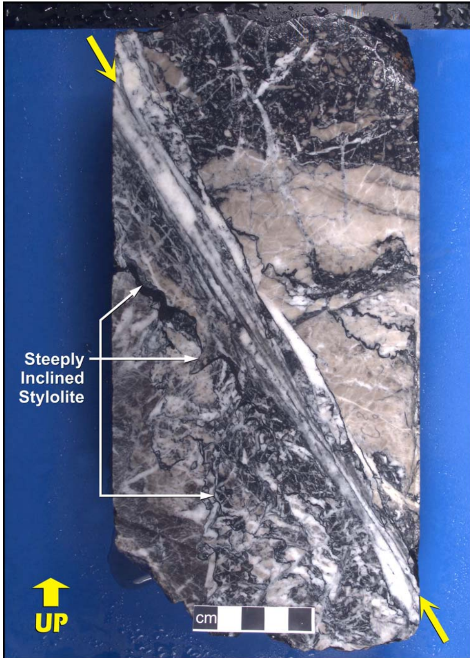
Interpreted thrust fault zone in the Blue Fiord Formation. The zone consists of multiple inclined parallel fractures (arrows), infilled by white equant calcite. Similar calcites infill other fractures, especially in the footwall of the thrust. Note the bitumen-infilled steeply inclined or near-vertical stylolites in the lower left part of the photograph. The presence of steeply inclined and near-vertical stylolites implies horizontal compression and is evidence supportive of thrust faulting. The position of this well lies in close proximity to the traces of thrust faults mapped from seismic by Panarctic Oils Ltd. Photograph taken of a wetted core surface. W. Bent Horn I-01, 10,675.95 ft.
