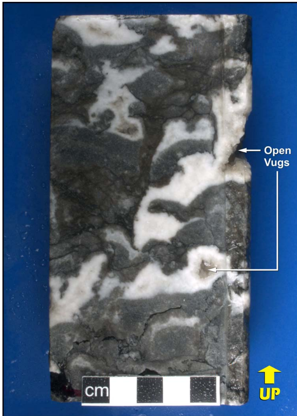
Core photograph of channel-form solution vugs with horizontal and oblique orientations. The peripheral portions of the vugs are infilled by white crystals of saddle dolomite, but the interior portions remain open. This full-diameter core segment has a porosity of 2.2% and a K_{\max} of 0.26 mD. Photograph taken of a wetted core surface. Muscox D-87, 2081.60 m.
