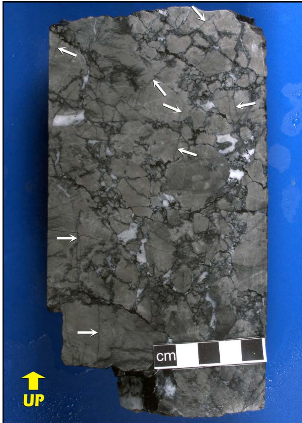
Core photograph of a matrix-rich clast-supported chaotic dolobreccia, but with some aspects of crackle and mosaic breccias. White coloured dolomite and calcite cements infill some sheltered pores that occur beneath breccia clasts. Bitumen infills narrow fractures (arrows) confined to the breccia clasts. Photograph taken of a wetted core surface. Kusrhaak D-16, 12007.5 ft.
