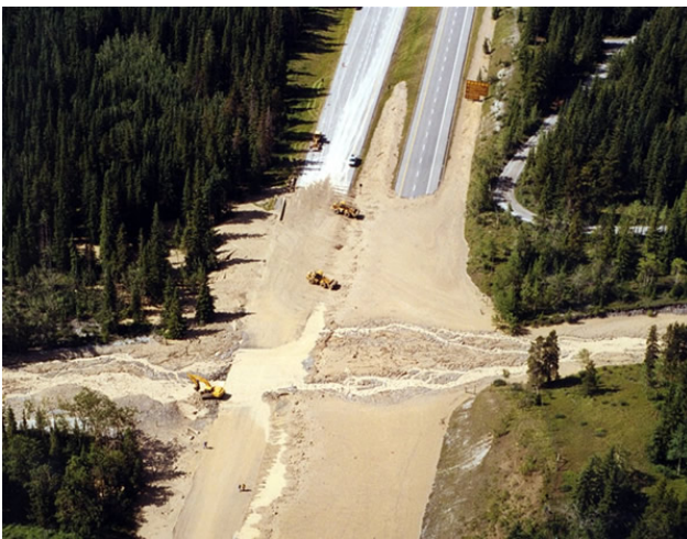
Figure 18. Five Mile Creek debris flow, Alberta. The August 1999 debris flow which covered the Trans-Canada Highway for 24 hours was unexpected and a result of intense rainfall.
