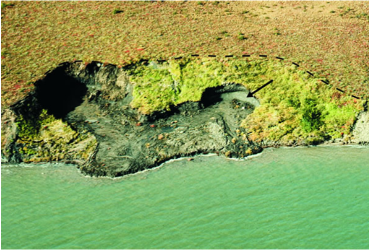
Figure 16. Retrogressive thaw flow in ice-rich sediment near Tuktoyaktuk, Northwest Territories. The flow is a reactivation within an older retrogressive thaw flow scar (dashed line indicates older scarp.) The colour change visible in the vegetation cover reflects the moister conditions occurring within the old scar. Massive ground ice (arrow) is visible in the new scarp.
