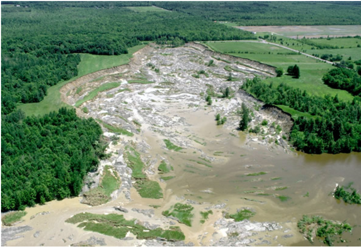
Figure 23. Lemieux Landslide, Ontario. Aerial view of the 1993 Lemieux landslide taken 4 days after the event. The flood waters of the South Nation River, which rose 12 metres to overtop the debris dam, have inundated the mouth of the landslide scar.
