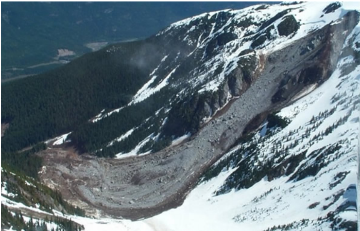
Figure 3. Zymoetz Landslide, British Columbia. A complex rock avalanche–debris flow that occurred on June 8, 2002, approximately 30 kilometres east of Terrace, British Columbia. The debris travelled for more than 4.5 kilometres, descending about 1250 metres. The landslide ruptured a gas pipeline, triggered a forest fire, dammed the Zymoetz River, flooded a Forest Service road and destroyed a bridge.
