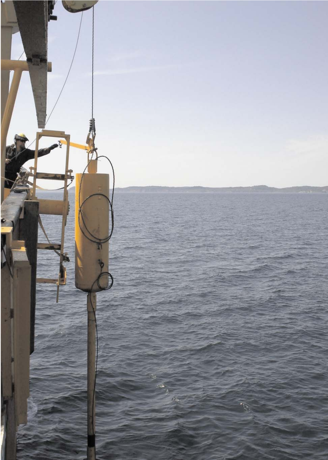
Figure 73. Piston corer being deployed off the starboard bow of the CCGS Hudson .
