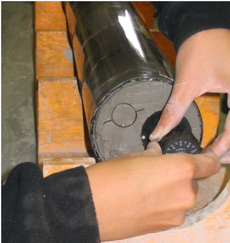
Figure 74. Taking a Torvane measurement.
