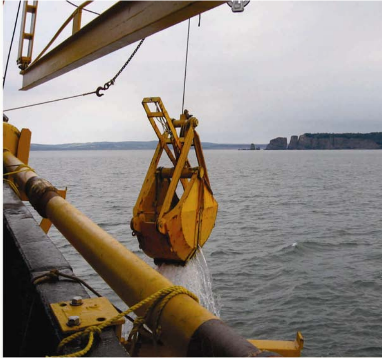
Figure 71. Large IKU grab sampler used for surface and shallow sub-surface sampling.
