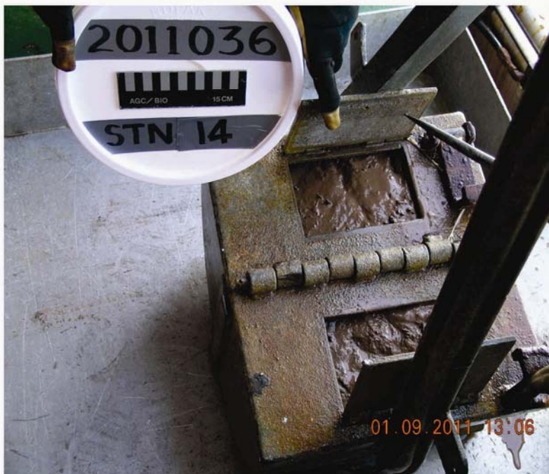
Figure 72. Medium size van Veen grab sampler.
