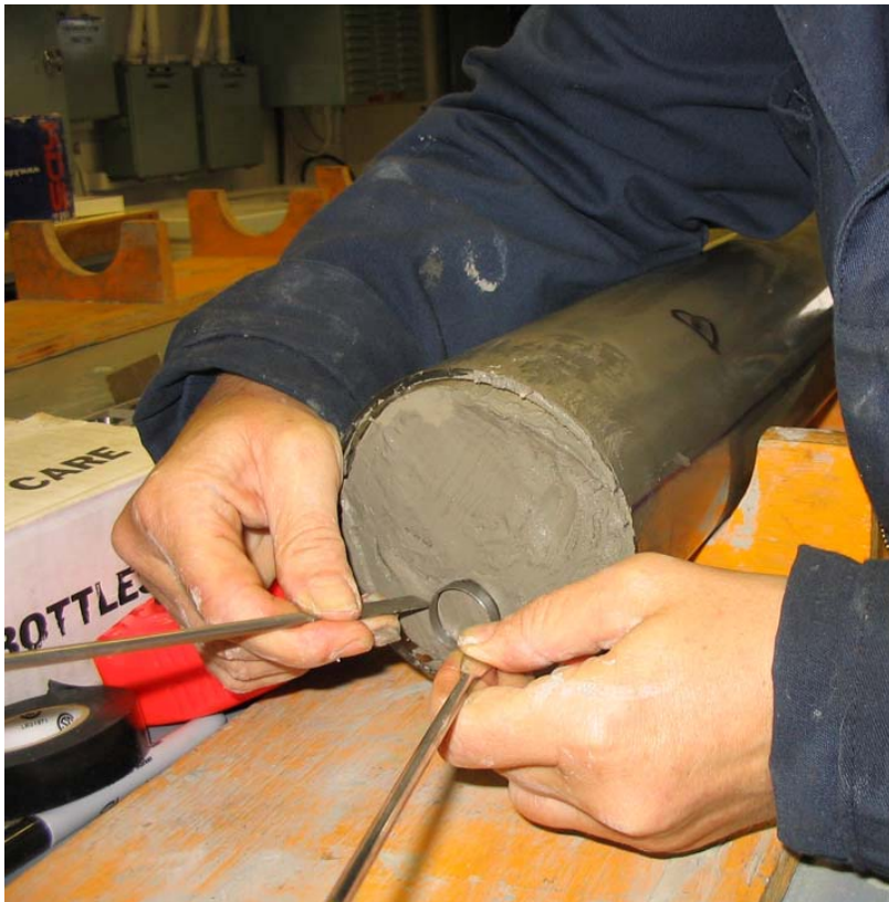
Figure 75. Inserting the constant volume sampler.
