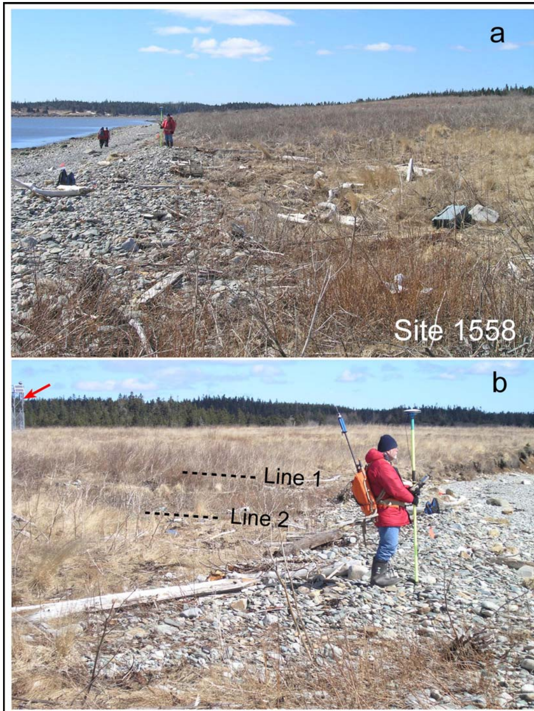
Figure 1558-1 Views looking alongshore at site 1558 (a) to the west and (b) east showing the location of survey lines and the navigation marker at site 1542. This low beach is often overwashed by waves as shown by the debris along the backshore in March 2011. Figure 1557-2 provides a more general view of the site location along the north shore of Louisbourg Harbour.
