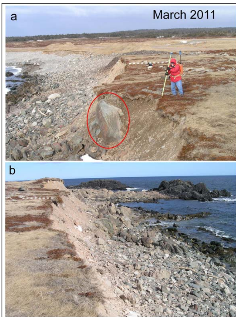
Figure 1532-3. Views of the cliff face at site 1532 looking (a) to northwest and (b) to southeast showing conditions in March 2011. Dashed line marks the survey line location.
