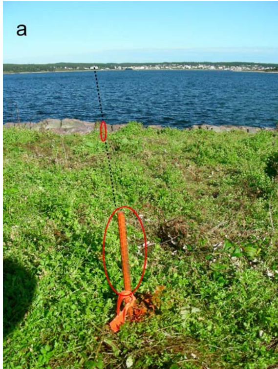
Figure 1561-1. Ground views at site 1561, Battery Island showing (a) line markers and alignment with peak at Point of View building in Louisbourg and views (b) east and (c) west alongshore with BM2 line marker (circled) in foreground. (Photos 26-Sept 2011).
