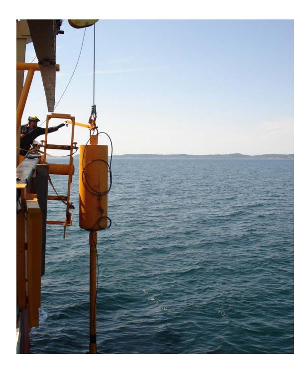
Fig. 4-3 Piston corer being deployed off the starboard bow of the CCGS Hudson. Photo courtesy of Brian Todd
