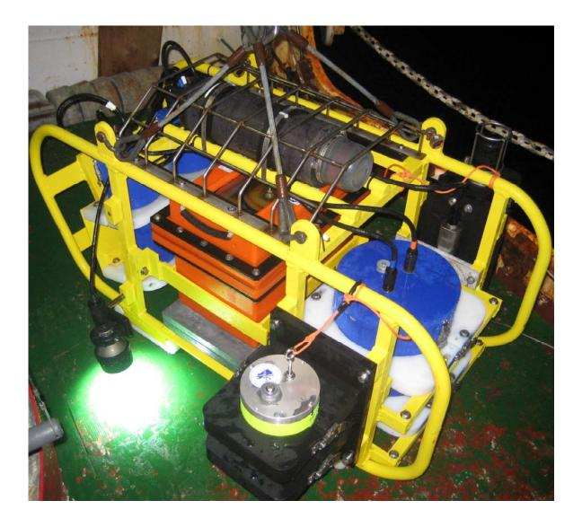
Fig. 4-4 Photograph of the 4K Camera System used in Hudson 2010020 mission.
