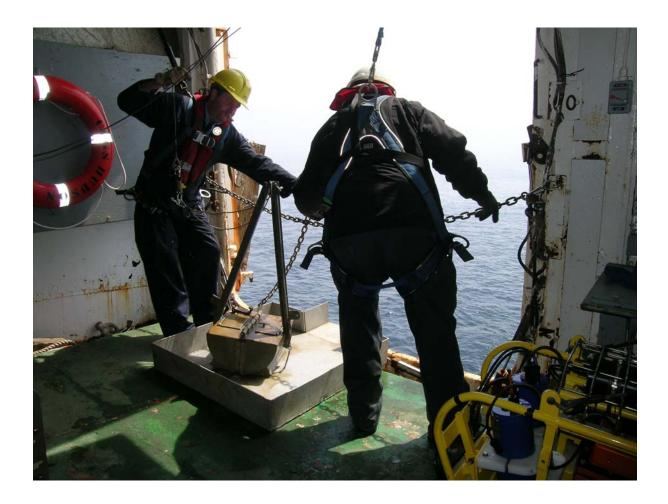
Fig. 4-1 Photograph of the van Veen grab sampler used in this cruise.
