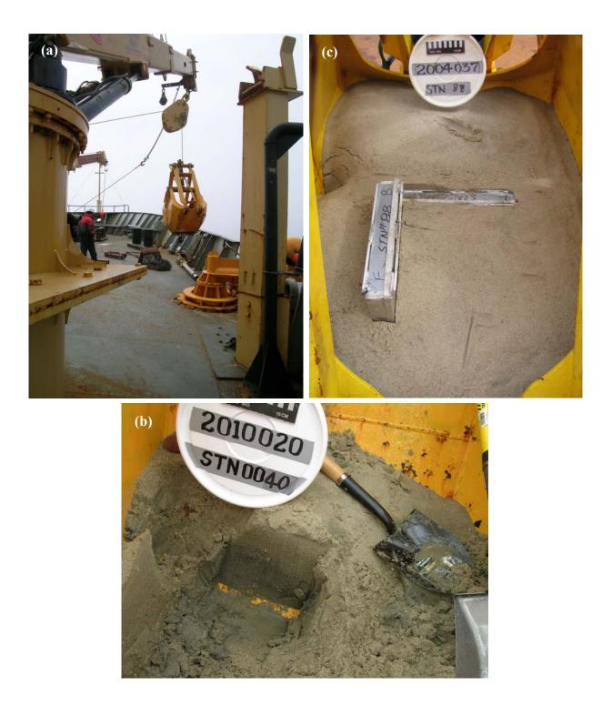
Fig. 4-2 Photographs of (a) the large IKU grab sampler used in this mission, (b) vertical profile cut into the IKU sample, and (c) box-core trays pushed into the IKU grab sample.
