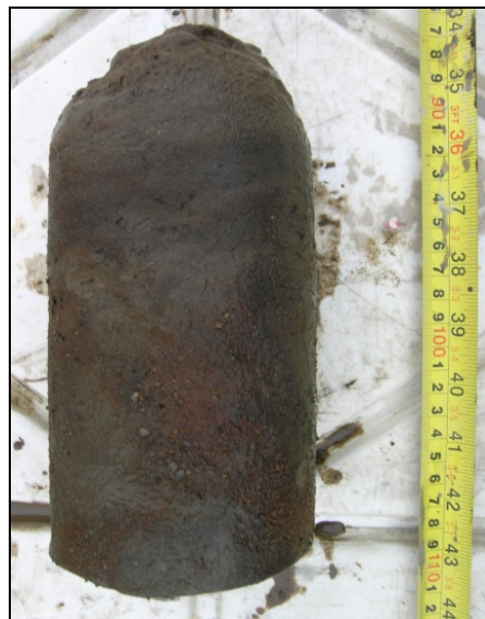
Figure 14: Permafrost core sample taken in an old alluvial channel (SDH-19). See Figure 2 for site location.
