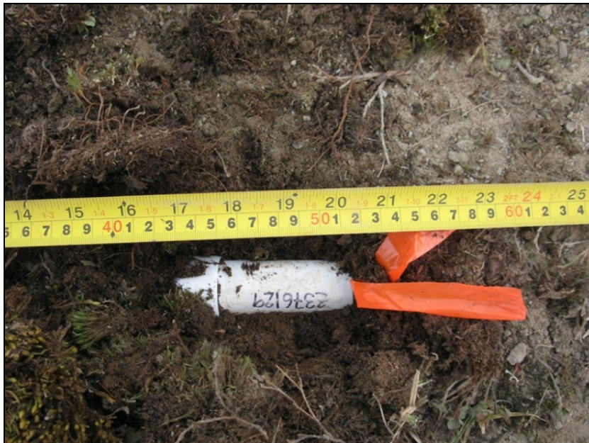
Figure 6: Miniature data logger (HOBO) used to record ground surface temperatures.
