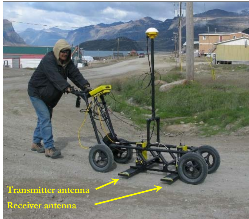
Figure 9: Ground penetrating radar (GPR) unit by Sensors and Software Inc. showing the antennas mounted on the cart.
