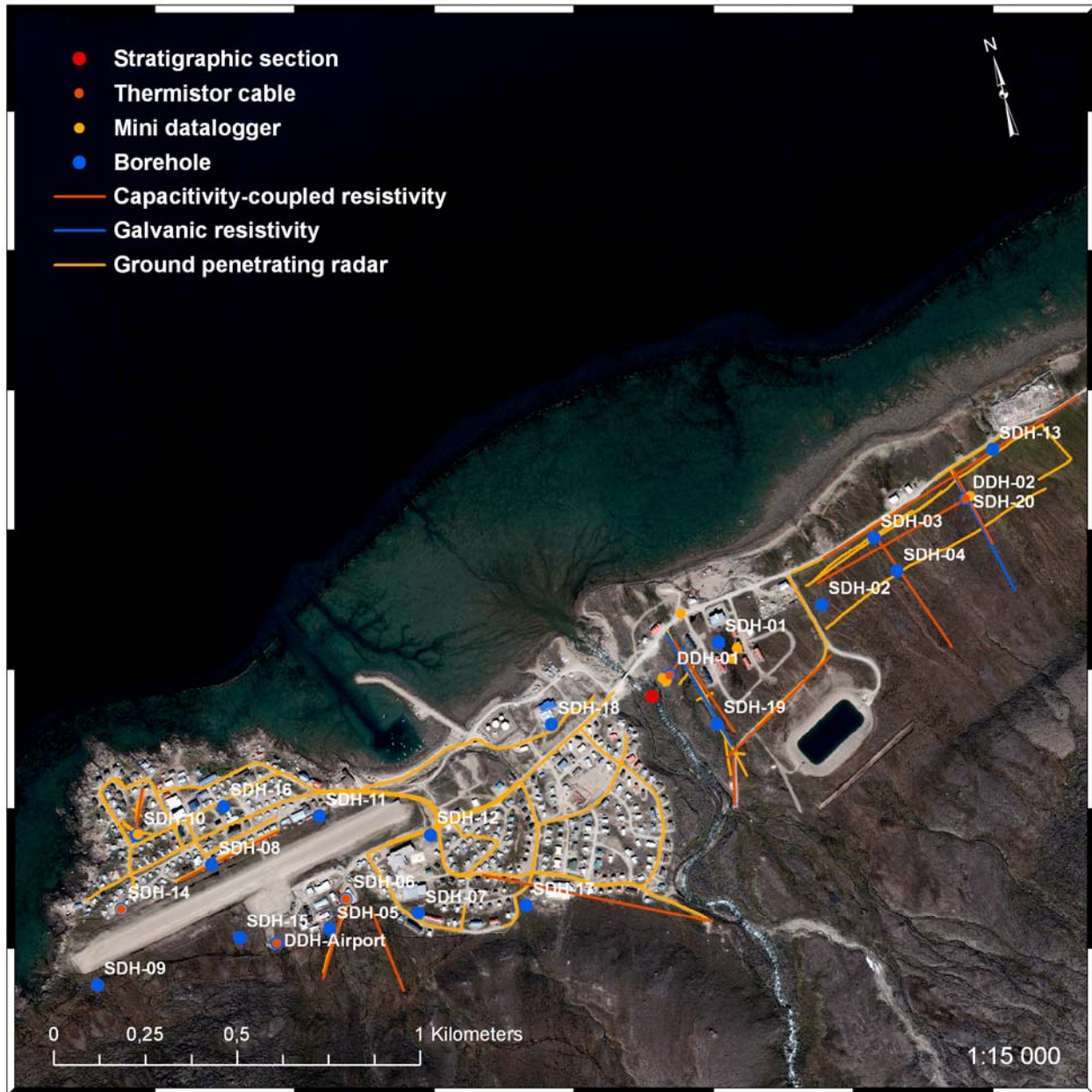
Figure 2: Summary of the summer 2009 field work. Location of boreholes, thermistor cables, air and ground surface temperature sensors and geophysical surveys. Background image (Quickbird), Includes copyrighted material DigitalGlobe, Inc., all rights reserved.
