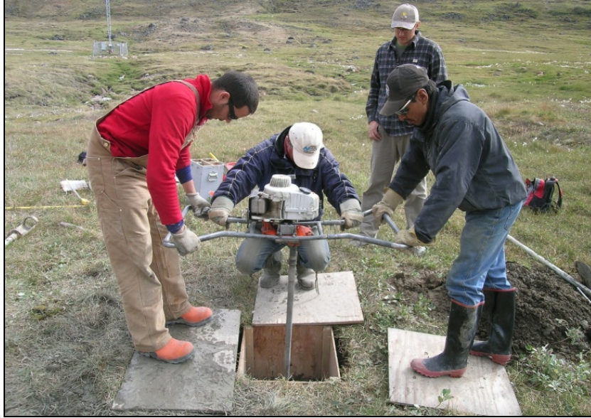
Figure 3: Shallow drilling with the portable earth drill.
