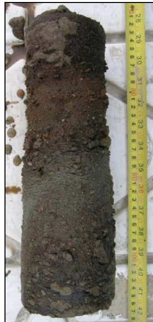
Figure 18: Permafrost core sample taken in the colluvial blanket (SDH-20). See Figure 2 for site location.
