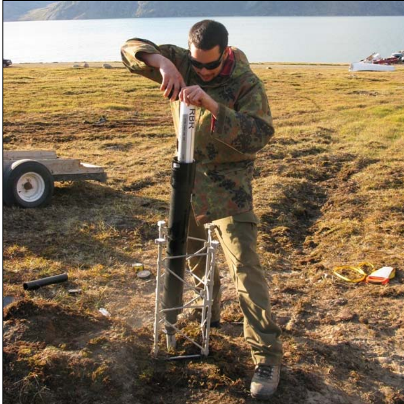
Figure 5: Thermistor cable and data logger in a PVC casing for permafrost temperature monitoring.
