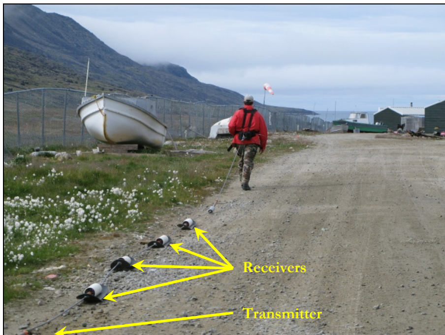
Figure 10: The capacively-coupled resistivity (CCR) OhmMapper composed of a coaxial-cable array with one transmitter and several receivers that are pulled along the ground.
