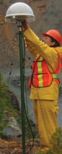
Setting up a GPS antenna for a temporary station near Myra Falls Mine on Vancouver Island. This region requires more detailed monitoring because it is close to the epicentre of the magnitude 7.3 Vancouver Island earthquake in 1946.
