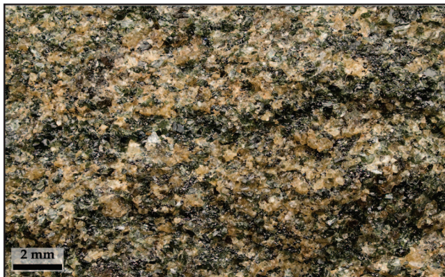
Figure 4. Relatively fine-grained peridotite M150 whose fresh surface exhibits abundant orthopyroxene and thin dark layers rich in olivine and chromite. 2011-184
