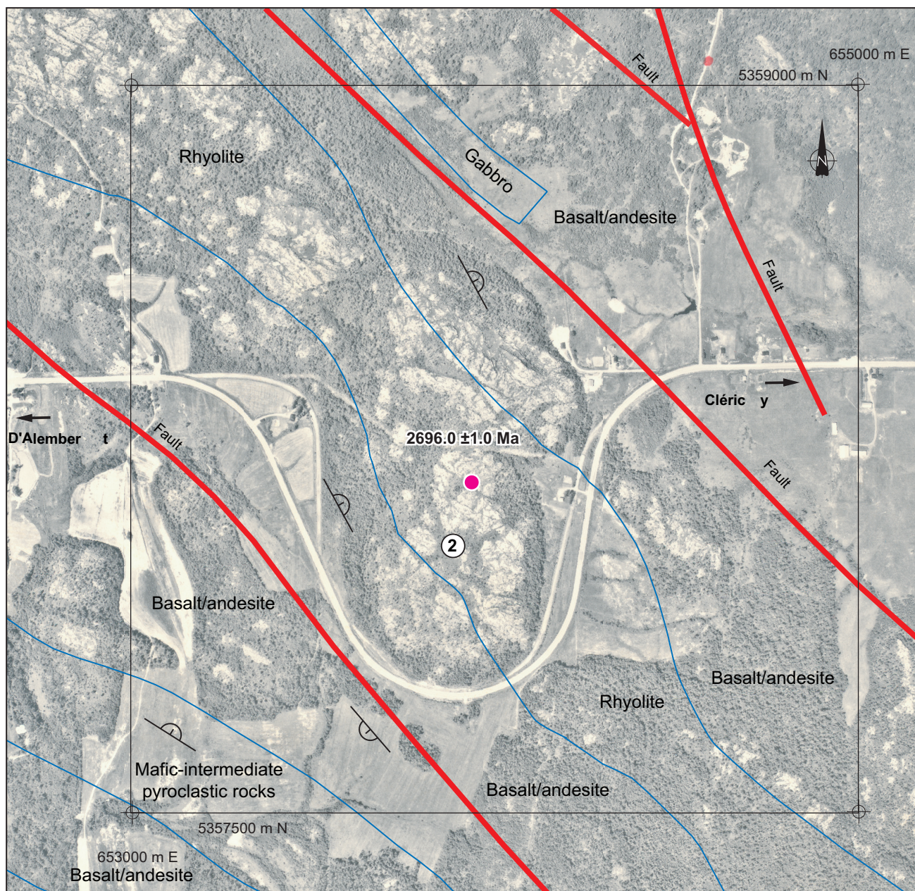
Figure 9. Aerial photograph showing the visited outcrop at stop 1-2, with the location of lithologic contacts.
