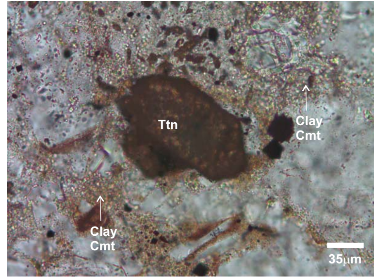
Figure 108a: 3074.30 m 50x (line 11): Titanite and clay cement (pp)
