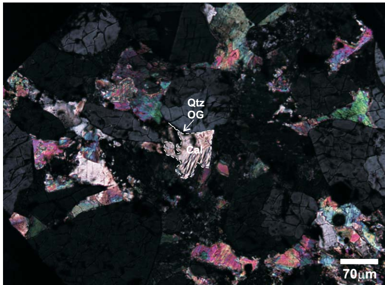
Figure 3b: 2465.18m 20x (L2): Late calcite in contact with quartz overgrowths (xpl)
