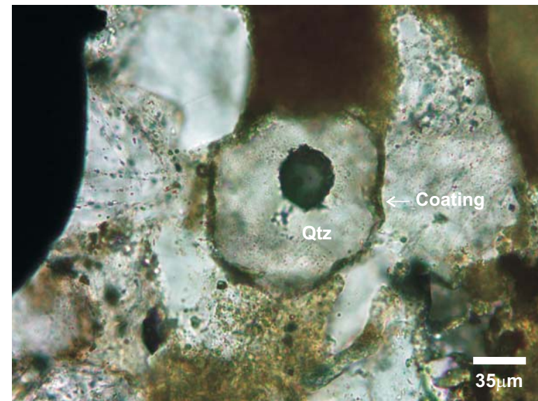
Figure 59a: 3024.35 m 50x (line 5): Detrital quartz with clay (detrital) coating (ppl)
