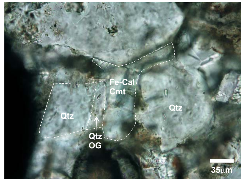
Figure 23a: 2494.36 m 50x (line 1): Late ferroan calcite cement in contact with quartz overgrowth (ppl)
