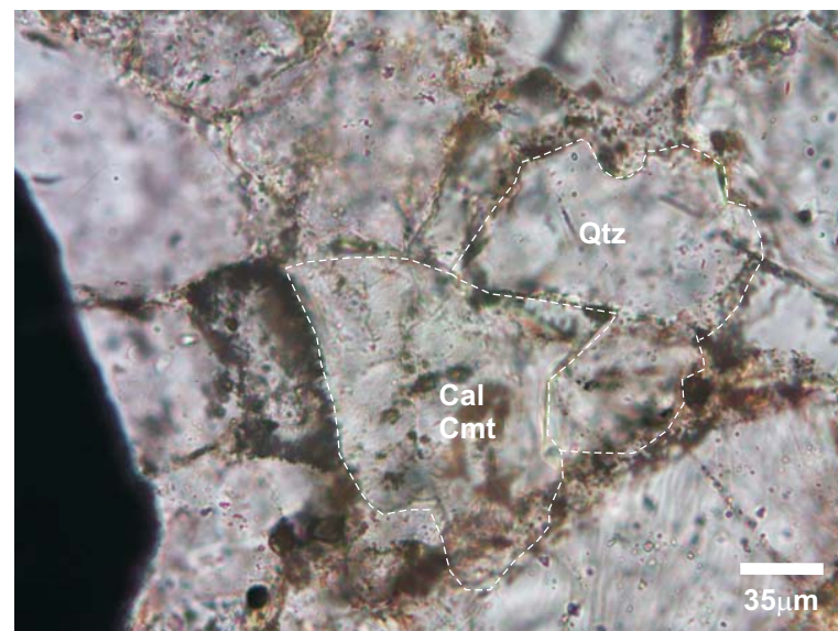
Figure 54a: 2934.50 m 50x (line 12): Early calcite in contact with quartz grains (ppl)
