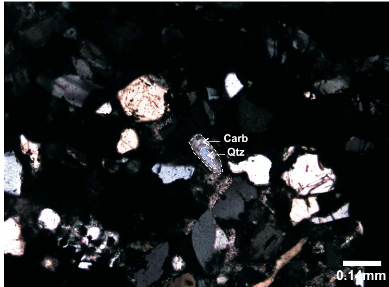
Figure 7b: 2466.37m 10x (L1): Microcrystalline carbonate engulfing detrital quartz (xpl)
