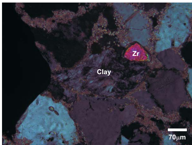
Figure 103b: 3074.30 m 20x (line 1): Clay intraclast (illite) and zircon (xpl)
