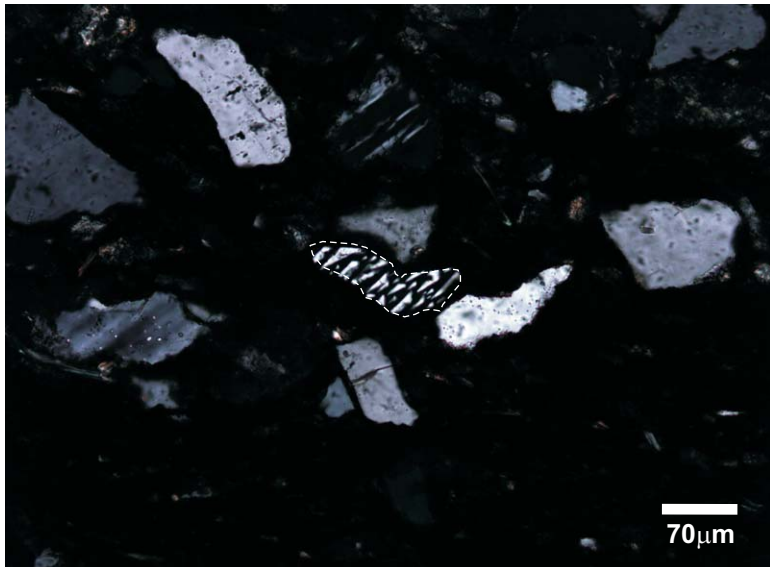
Figure 6b: 2474.79m 20x (L5): Lithic clast with graphic texture (xpl)
