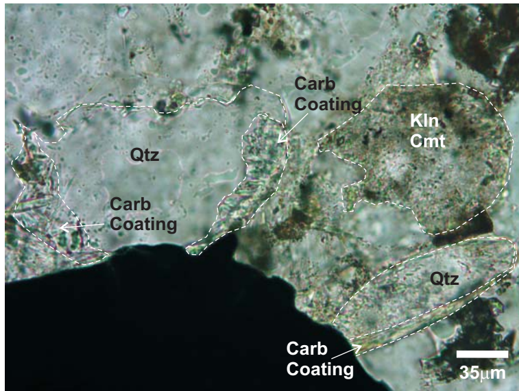
Figure 101a: 3068.40 m 50x (line 2): Two quartz grains engulfed by carbonate, and uncompact kaolinite cement (ppl)
