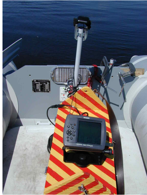
Close up view of the GPS receiver and sonar fish finder.
