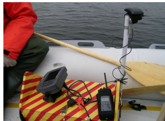
Equipment used for collecting bathymetric data: Sonar fish finder and GPS receiver.
