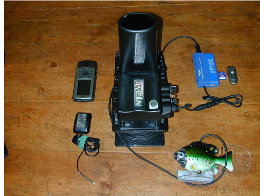
Underwater video camera equipment used to observe T-Lake intake pipe.
