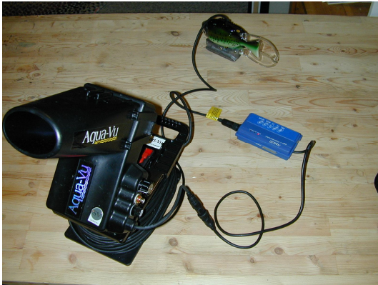
Underwater video camera equipment used to observe T-Lake intake pipe.
