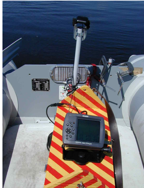
Close up view of the GPS receiver and sonar.
